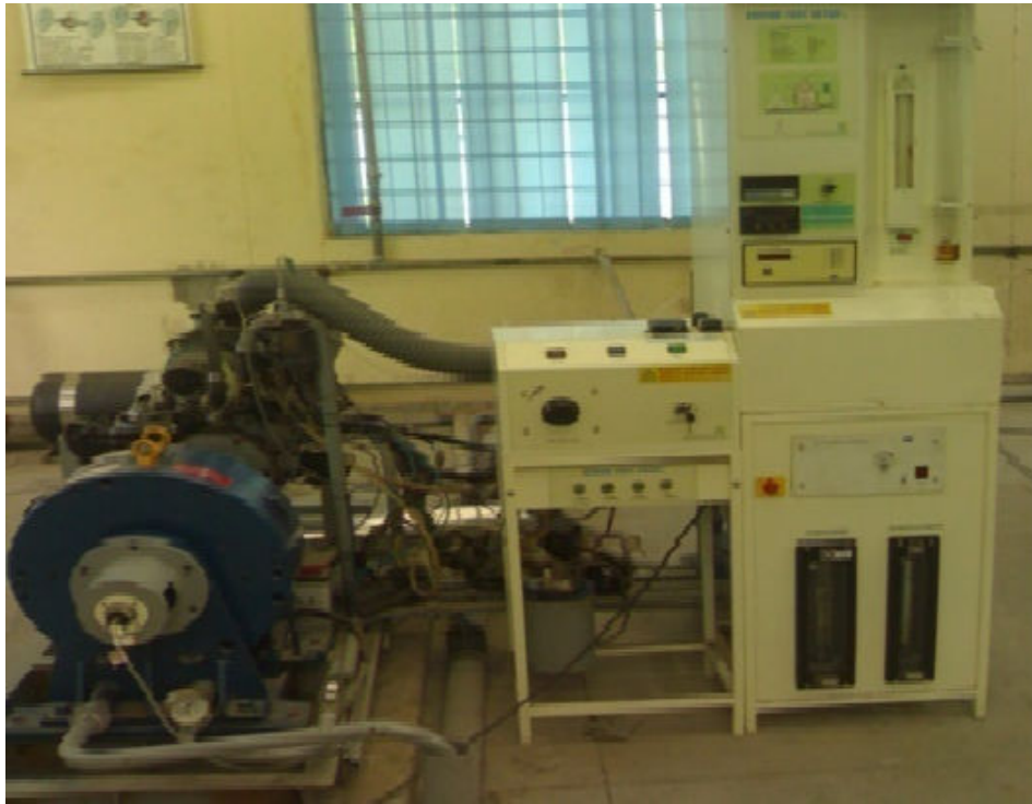
Figure 7.2: The Actual Test Set-up of Maruti Wagon (R) MPFI Engine
