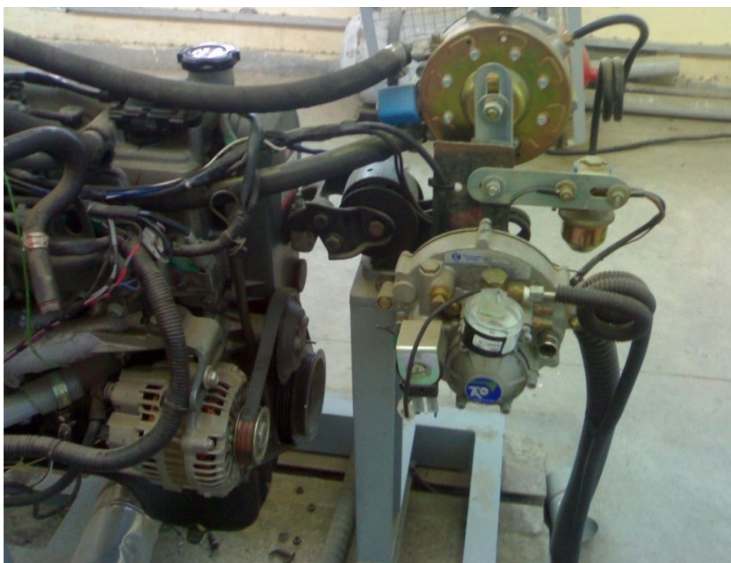
Figure-7.6 LPG and CNG Conversion Kits Mounted on the Engine
