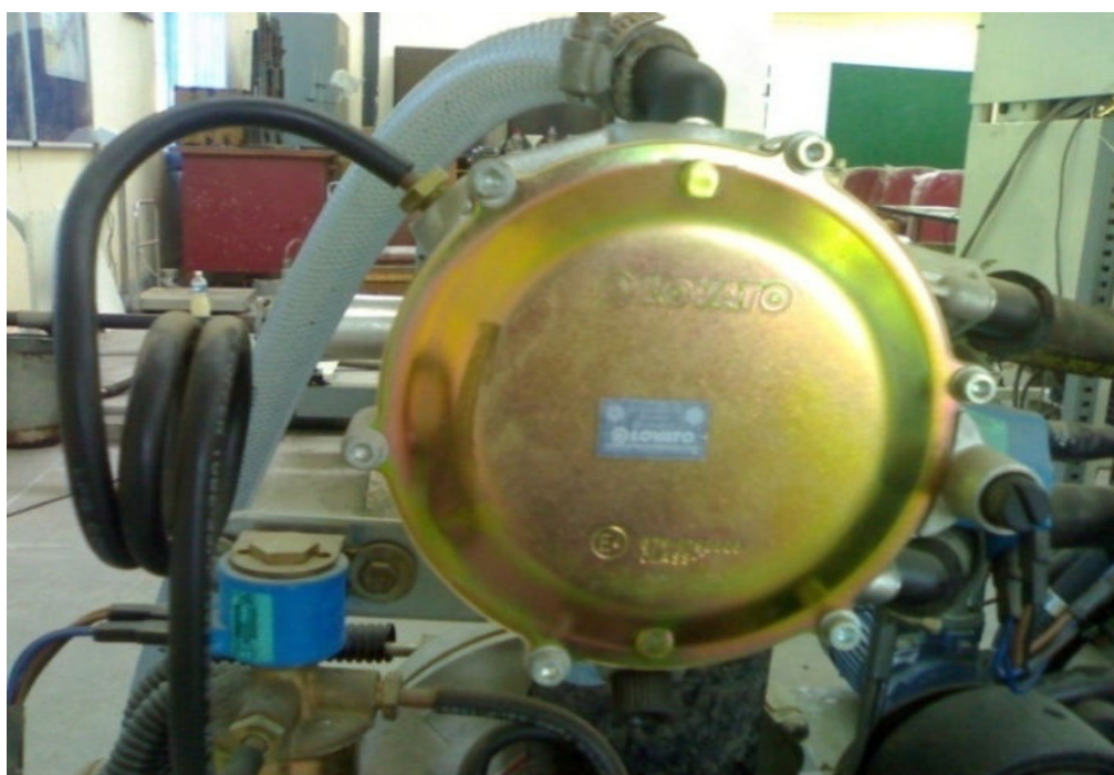
Figure 7.5: The LPG Conversion Kit–Pressure Regulator
