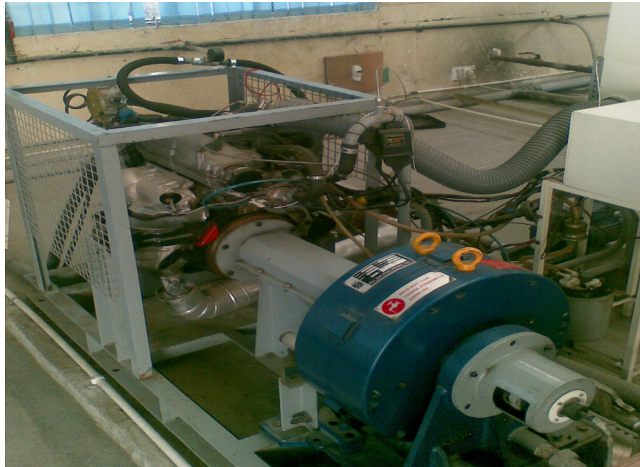
Figure 7.3: Wagon R Engine Coupled to the Eddy Current Dynamometer
