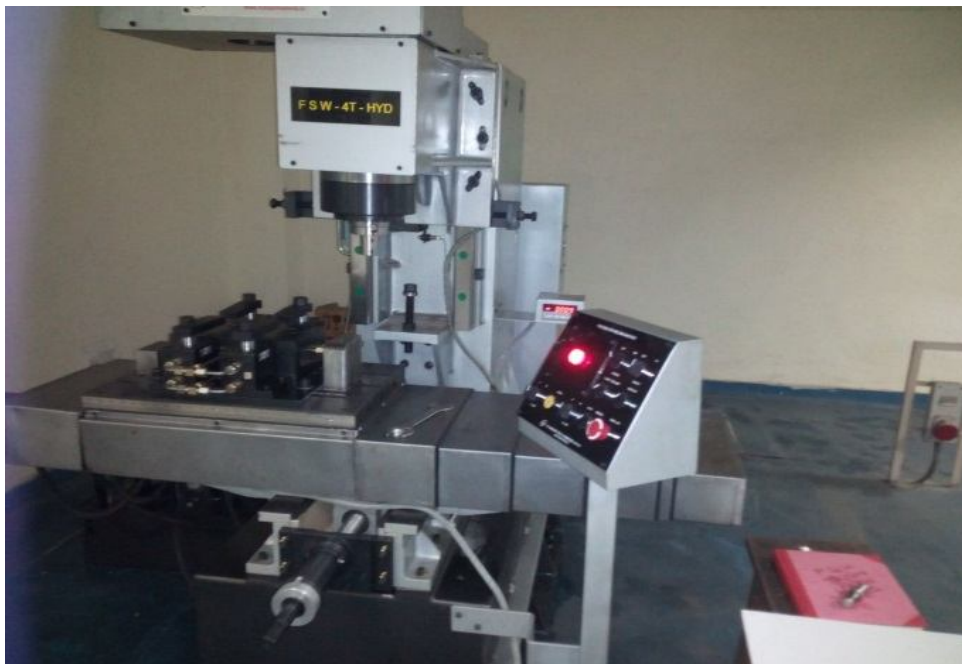
Fig. 2: Friction stir welding / processing machine (Central workshop, Delhi Technological University)
