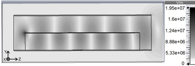
Fig. 10. Simulated electric field inside the mode converter with SF_6 medium in place of air and the corresponding color map.
