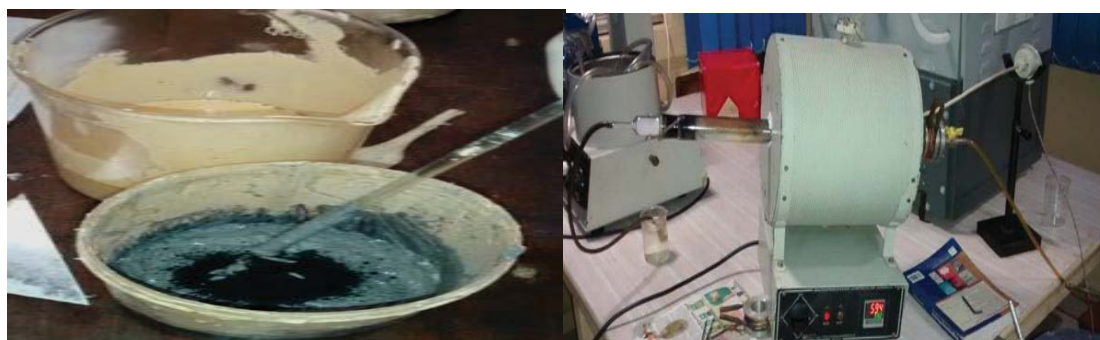
Fig. 1:- Abrasive laden Media (carrier+Al 2 O 3 +CNT) Fig.2. Thermal CVD Setup Fe-filled CNTs.
