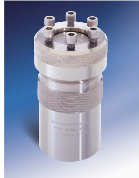
Fig. 15. Parr bomb (courtesy of Parr Instruments Company).
