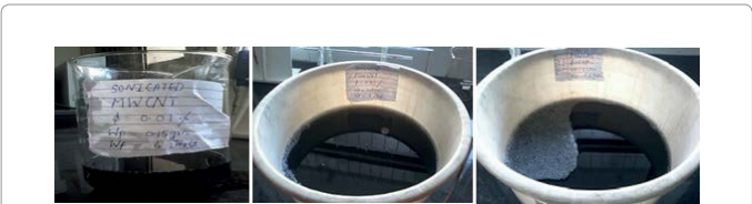
Figure 3: Sample of mixture ( \phi_v = 0.01\% ) and bucket of MWCNT nano fluids at 0.01% and 0.02% volume concentration.
