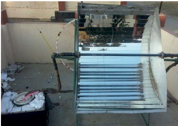
Figure 4: Parabolic trough collector (location: Thapar university).
