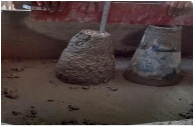
Fig.1 Workability measured by slump test
