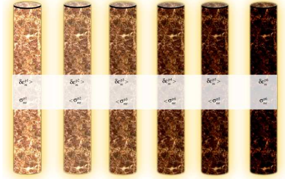
Fig. 6. The evolution of hardening and damage in six stages as an effect of accumulated plastic strains in hardening range to increase strength at all possible values of modified joint factor at selected RQDs.
