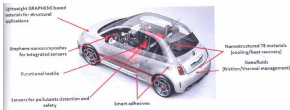
Fig. 5: Future Potential Application of Graphene in Automobiles
