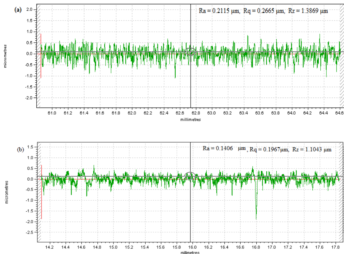
Fig. 5. (a) Surface roughness profile before finish; (b) Surface roughness profile after finish using bidisperse MRP fluid (sample 3)
