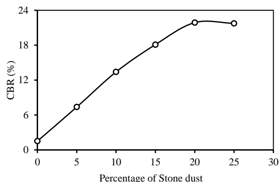
Fig. 4 Variation of CBR with percentage of Stone Dust in soil-lime (=9%) mix
