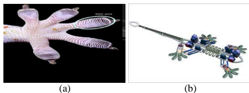
Figure 1. (a) Gecko feet, and (b) Sticky-bot: Gecko inspired wall climbing robot [1]
