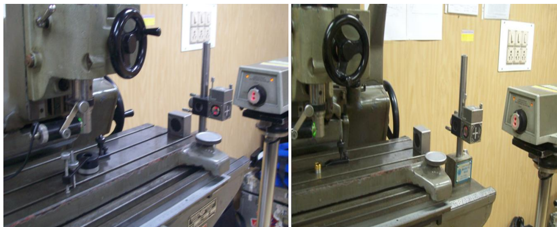
Fig. 2. Pictorial view of Universal Measuring Machine for measuring diameter of coupler (LHS) and the front cavity depth (RHS).
