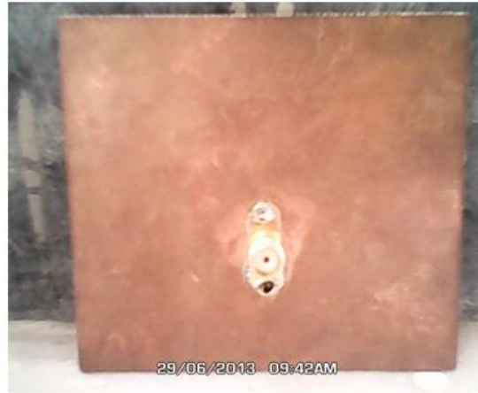
Figure 6. Bottom view of fabricated re-configurable fractal antenna
