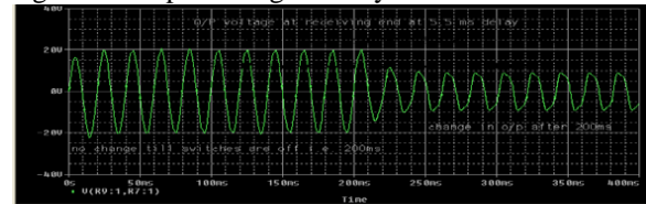
Figure 9. Out put voltage at delay of 5.5 ms
