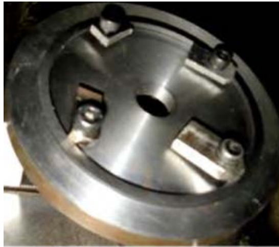
Fig. 1—Fixture with a clamped piston ring
