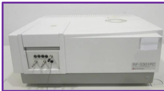
Fig.2.7. Shimadzu RF-5301 PC spectrofluorophotometer with a Xenon (150 W) bulb.
