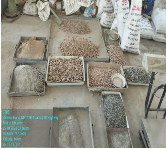
Figure 4.7 Sample Used for Filter media test
