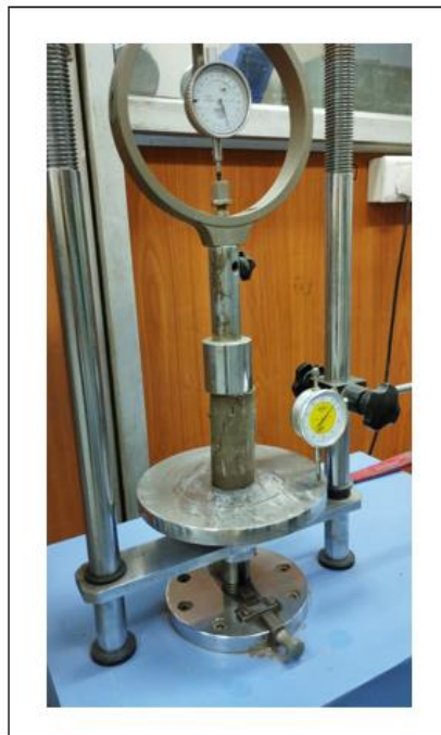
Fig 3.14: UCS on soil sample with 0% cement content
