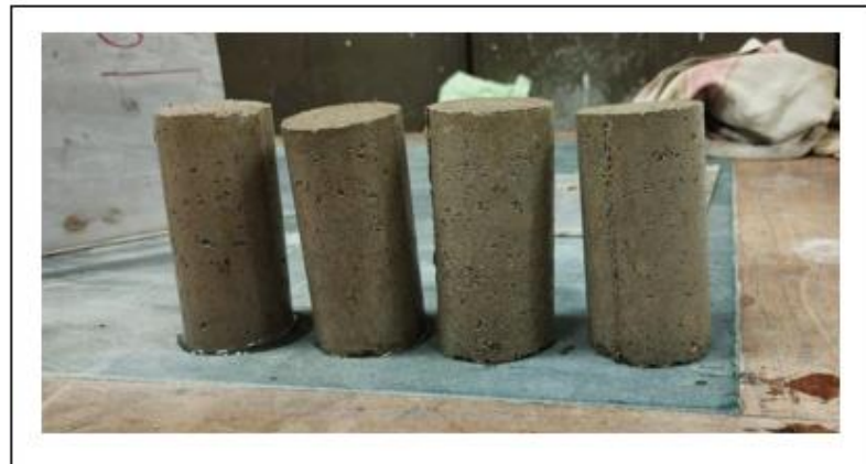
Fig 3.15: Samples with different percentage of cement (i)unsoaked (ii) soaked condition
