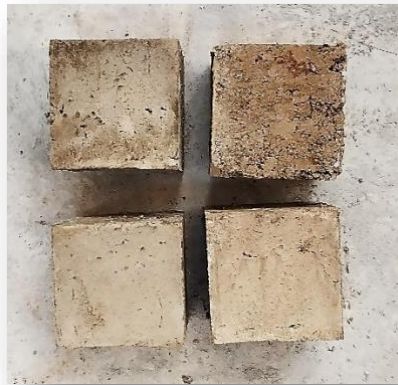
Fig 3.12: Cement stabilized cubes with varying %
