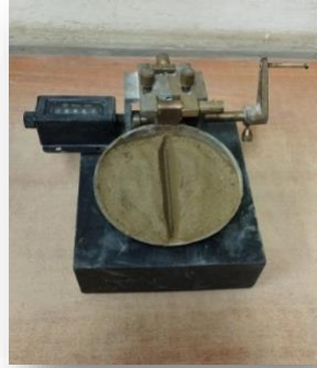
Fig 3.6: Casagrande's apparatus with soil sample
