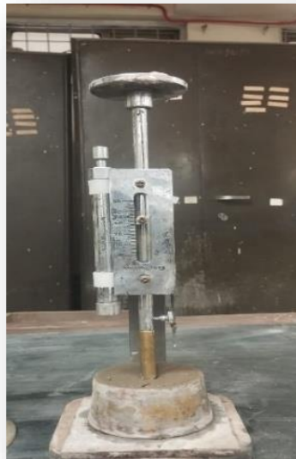
Fig 3.11: Normal consistency for soil cement mix
