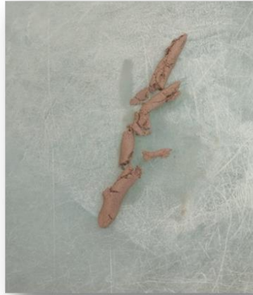
Fig 3.8: Crumbled thread of 3mm diameter
