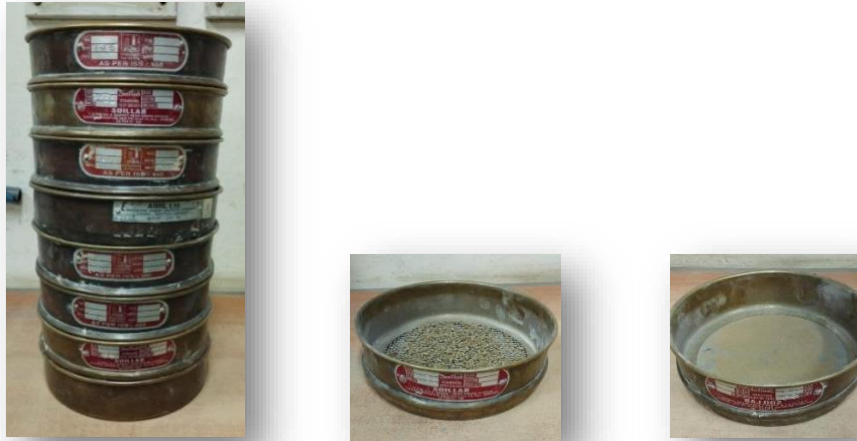
Fig3.2: Sieve analysis of soil sample
