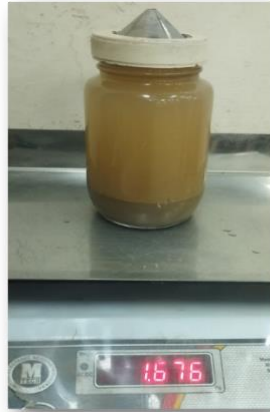
Fig3.1: Pycnometer with soil and water
