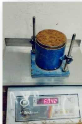
Fig 3.4: Standard Proctor Test mould
