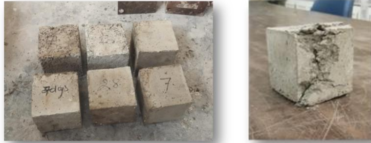
Fig 3.10: Casted cubes before and after testing
