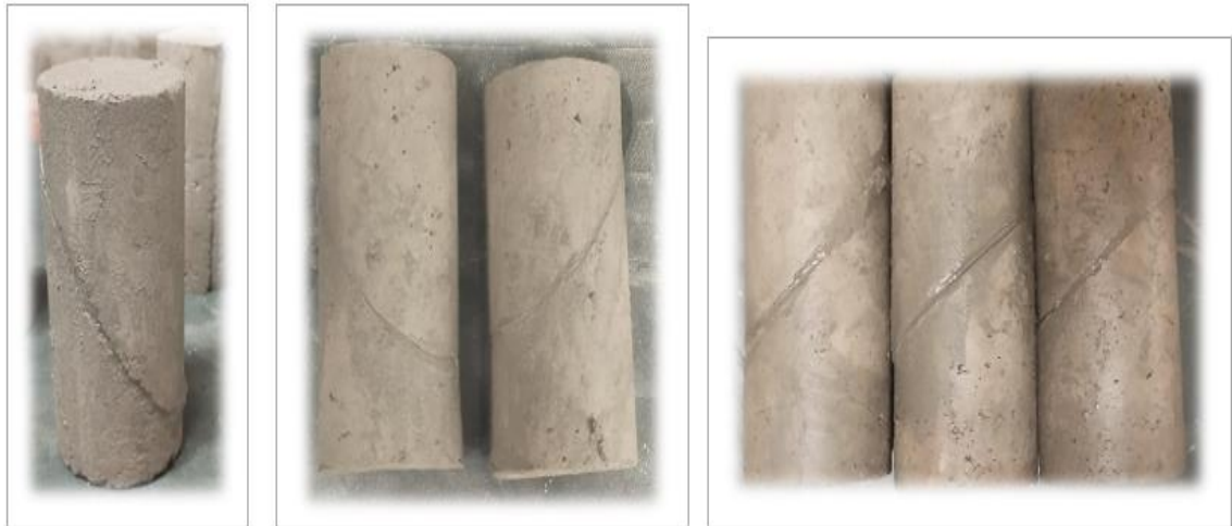
Fig 3.18: Grouted modelled rock 60°,45°,30° respectively
