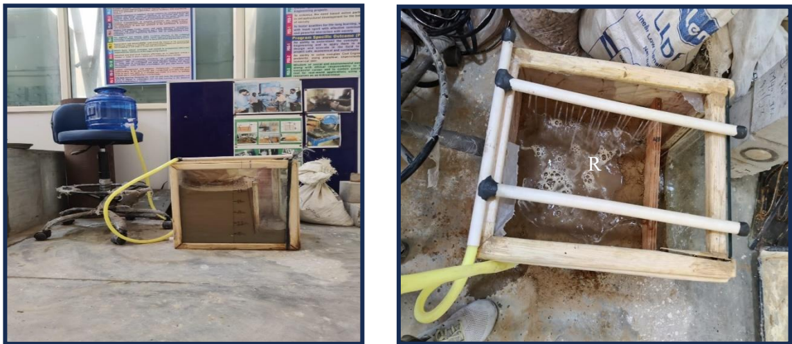
Figure 4.7 Reinforced Soil Earth Wall Experimental Model under Rainfall
