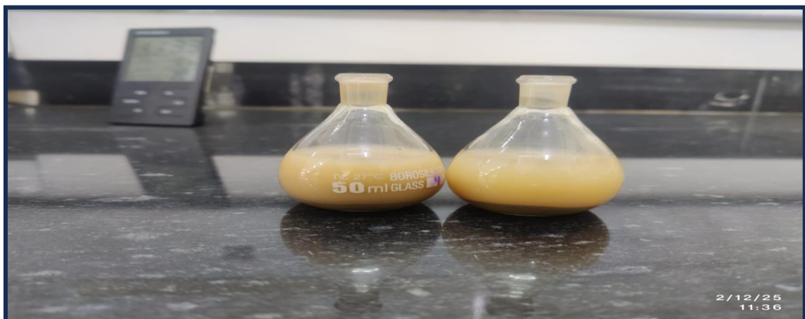
Figure 4.3 Density Bottle Apparatus Used for Determination of Specific Gravity of Soil
