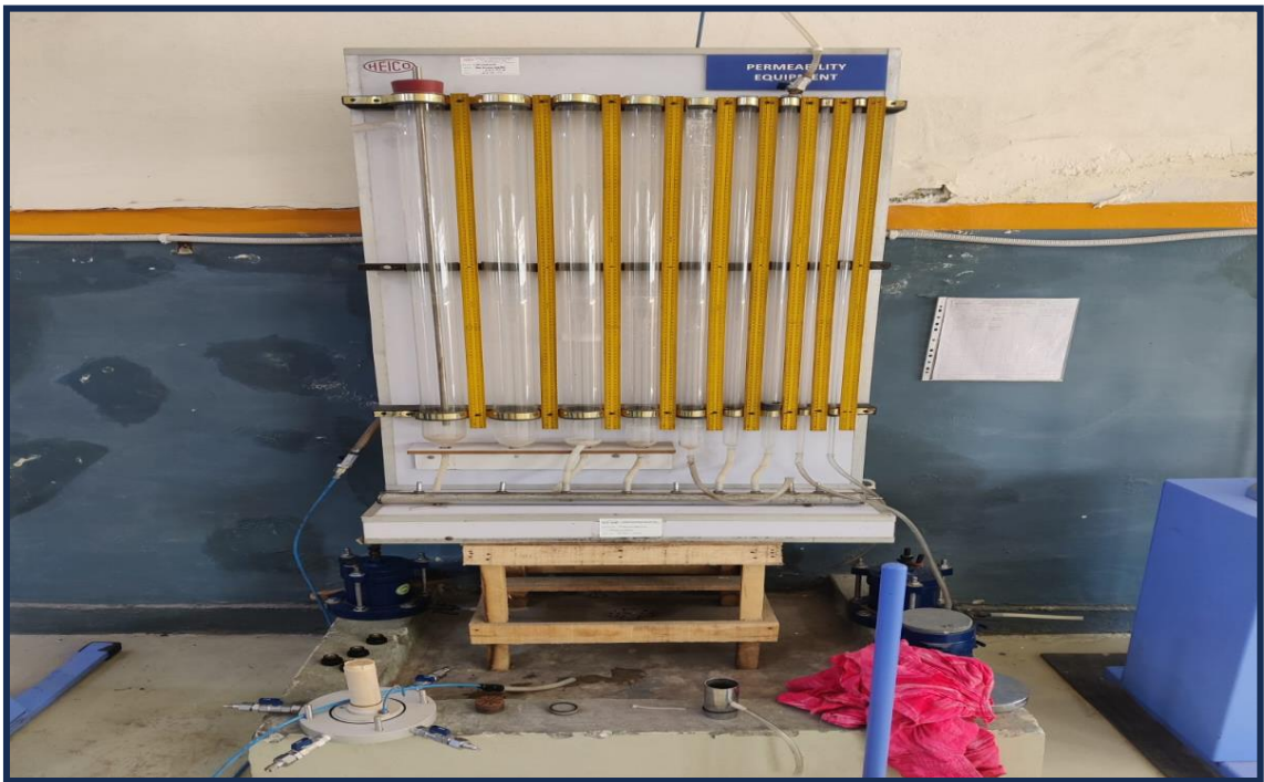
Figure 4.5 Permeability Apparatus Used for Determination of Coefficient of Permeability
