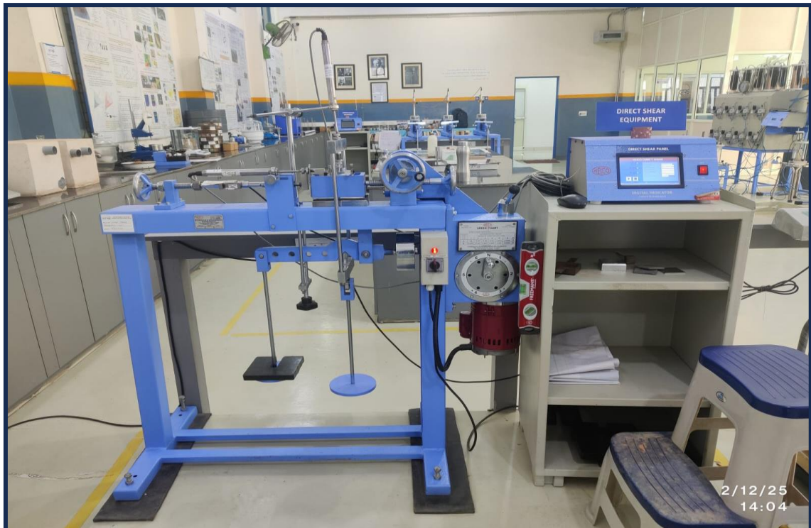
Figure 4.6 Direct Shear Test
