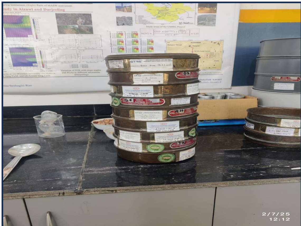
Figure 4.2 Standard Set of Sieves Arranged in Descending Order of Size for Grain Size Distribution Analysis
