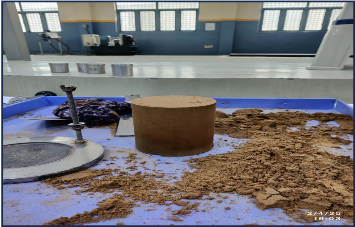
Figure 4.4 Modified Proctor Test Setup for Determination of Maximum Dry Density and Optimum Moisture Content
