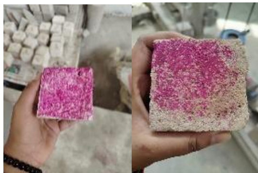
Figure 4. 8 Carbonation at the age of 28 days and 90 days
