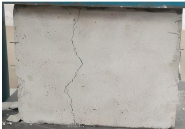
Figure 4. 3 Failure of cube due to compressive loading
