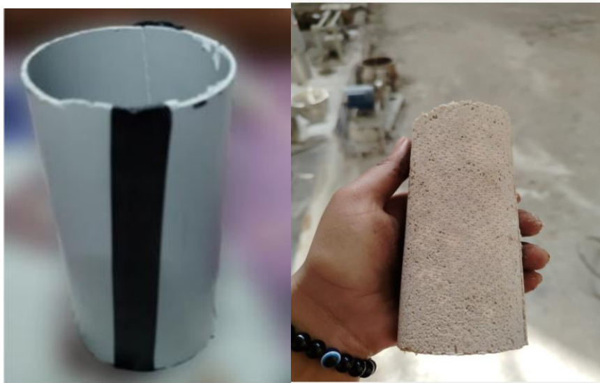
Figure 3. 5 Cylindrical mould and specimen for tensile strength test
