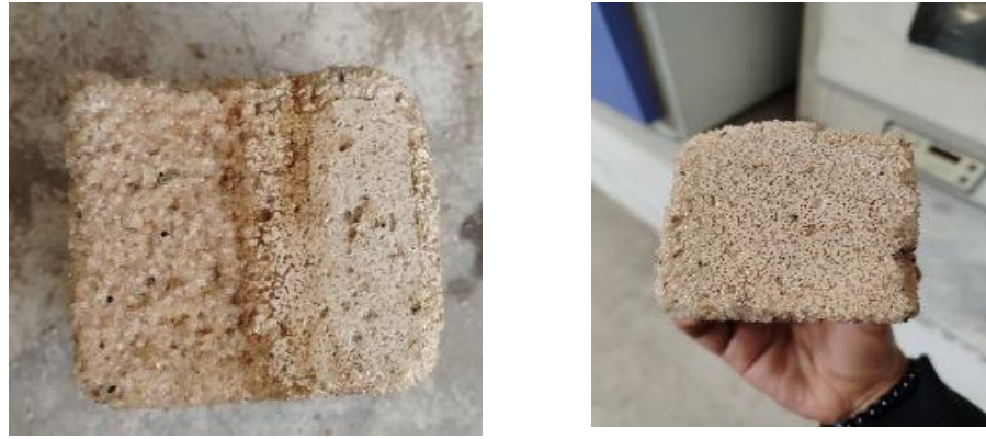
Figure 3. 7 Surface deterioration due to acid attack
