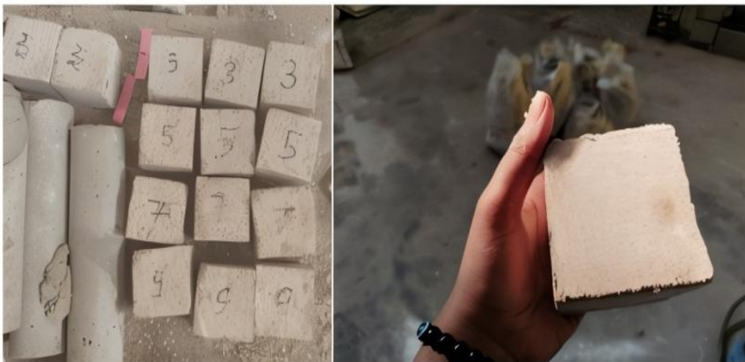
Figure 3. 3 Specimen for optimization of sticky rice
