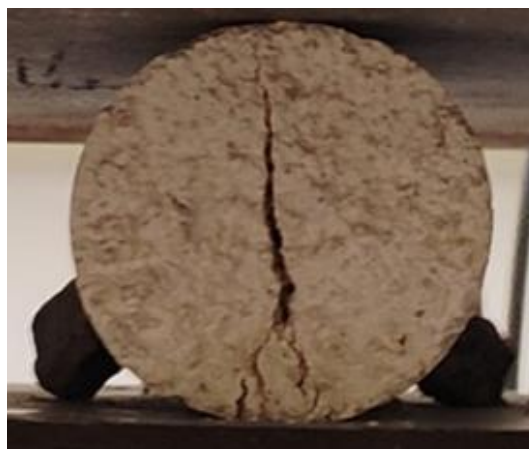
Figure 4. 6 Failure of cylindrical specimen
