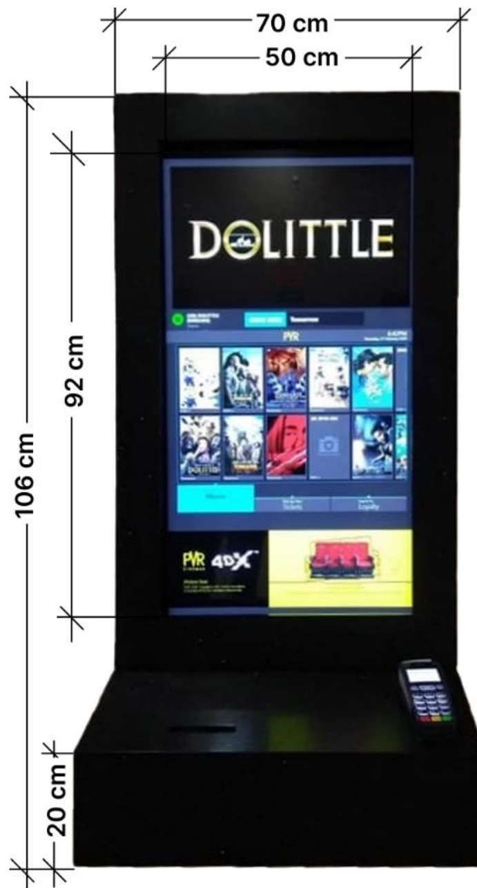
Figure 2: Dimension of PVR movie ticket machine
