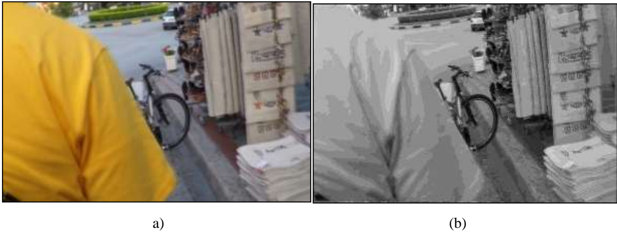
Figure 4.10: (a) Blurred image from the GoPro dataset, (b) Corresponding deblurred image after applying the Wiener filter.
