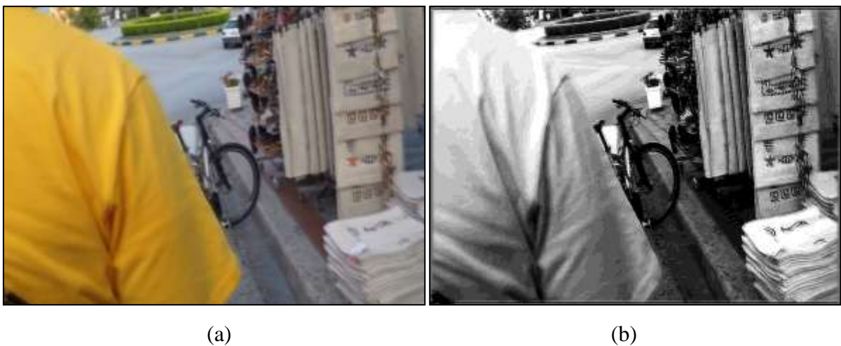
Figure 4.12: (a) Blurred image from the GoPro dataset, (b) Corresponding deblurred image obtained by applying the Lucy-Richardson deblurring algorithm followed by histogram equalization.
