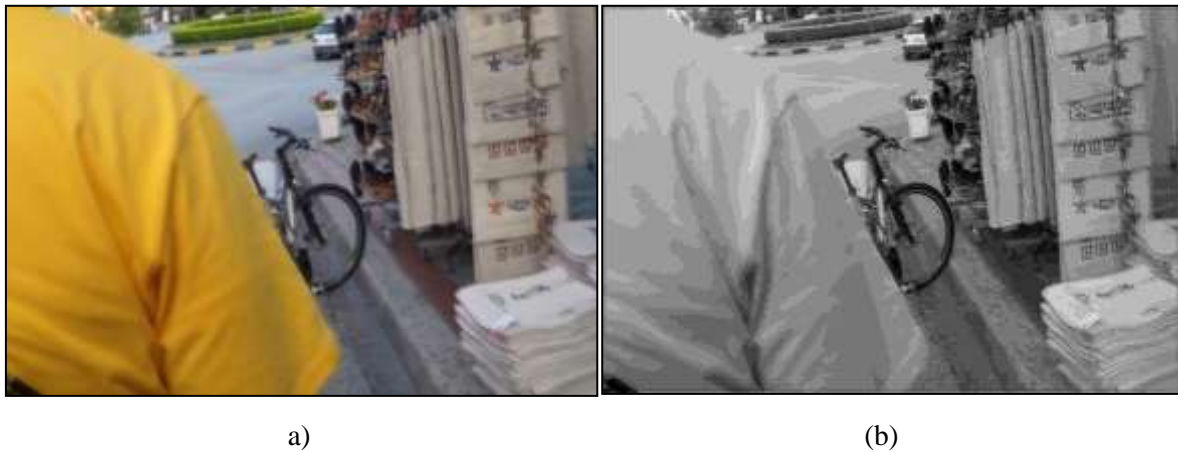
Figure 4.11: (a) Blurred image from the GoPro dataset, (b) Corresponding deblurred image after applying the Lucy-Richardson deblurring algorithm.
