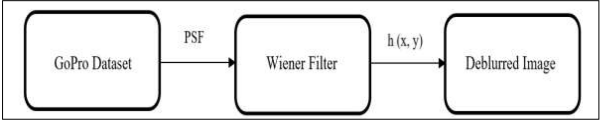
Figure 4.13: Workflow of the Wiener filter applied to produce a deblurred image.
