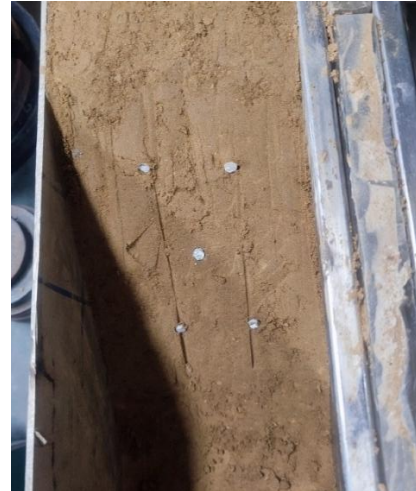
Figure 5.9: Staggered (Triangular) Nail Pattern
