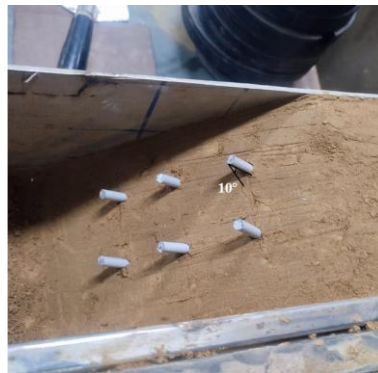
Figure 5.4: Aluminium solid tubes of 0.08m inserted at 10° to horizontal plane
