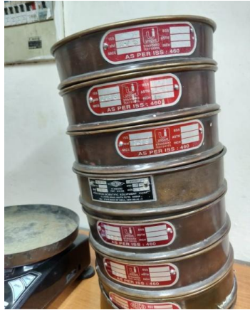
Figure 3.5: Sieve analysis arrangement
