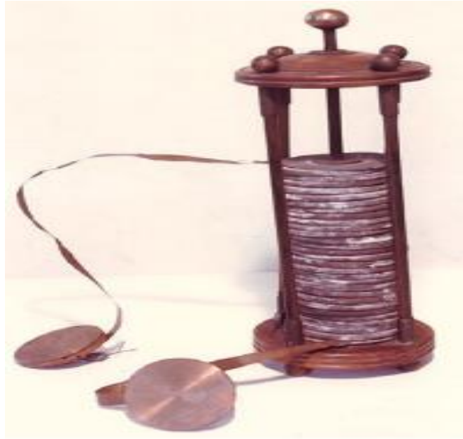
Fig.1.1 Electrical energy generation from a "galvanic cell" constructed through an alternating arrangement of two distinct metals (zinc and silver discs) isolated by a fabric immersed in a sodium chloride electrolyte
