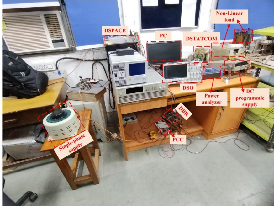
Fig 4.13 Experimental setup of single phase DSTATCOM
