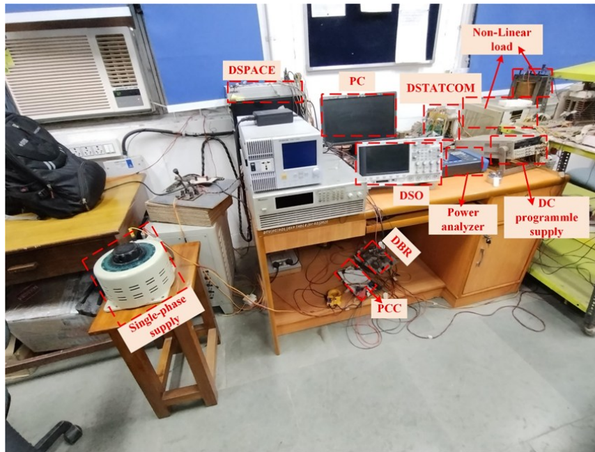
Fig 3.7 Experimental setup of single phase DSTATCOM
