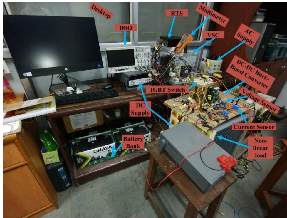
Fig. 6.9 Experimental setup up single phase grid interfaced EV charging systems
