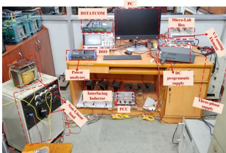
Fig 4.42 Experimental setup of three phase DSTATCOM
