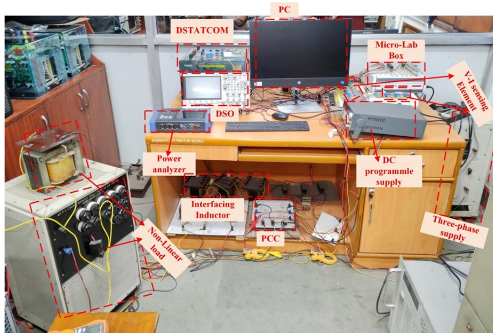
Fig 3.9 Experimental setup of three phase DSTATCOM
