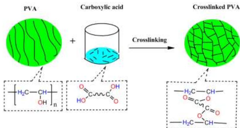
Fig. 1.1: Method of preparation of carboxylic acid crosslinked PVA
