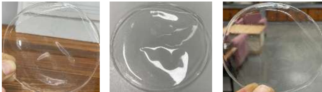
Fig. 5.1: Photographs of carboxylic acids crosslinked films: (a) Malonic acid crosslinked films; P-MA (b) Citric acid crosslinked film; P-CA (c) 1,2,3,4-tetracarboxylic acid crosslinked film; P-BTCA.
