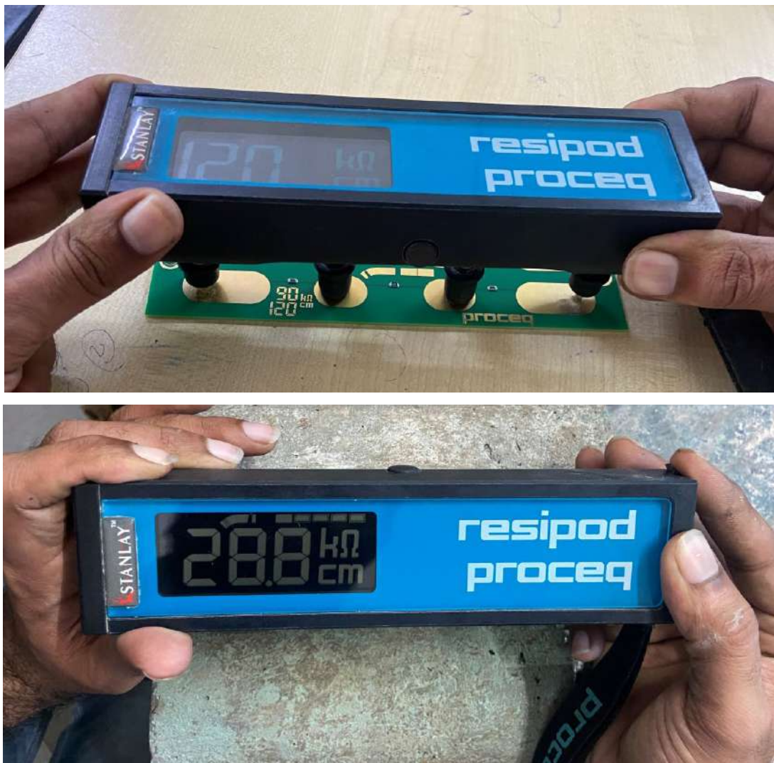
Figure 3.16 Resipod meter and a specimen under testing
