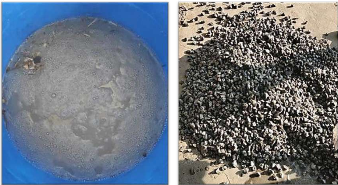
(a) Pre-soaking of RCA in acid
