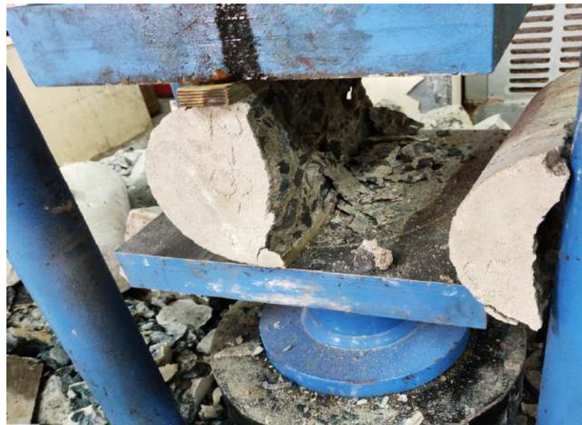
Figure 3.13 Split tensile strength determinations
