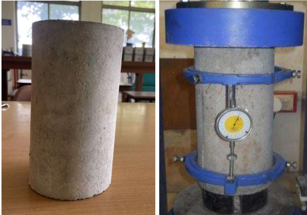
Figure 3.14 Modulus of elasticity determination
