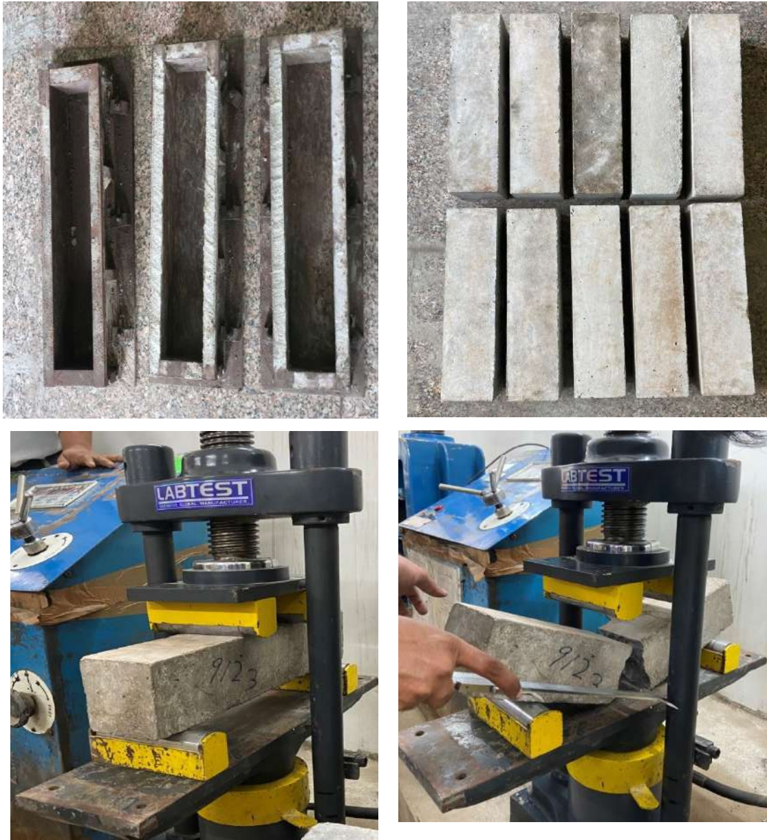
Figure 3.12 Flexural strength determination
