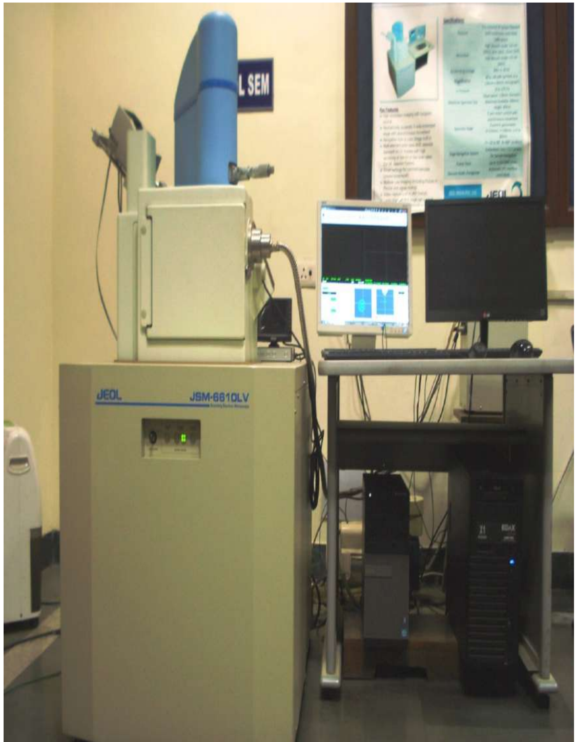
Figure 3.10 High resolution JSM 6610V scanning electron microscope
