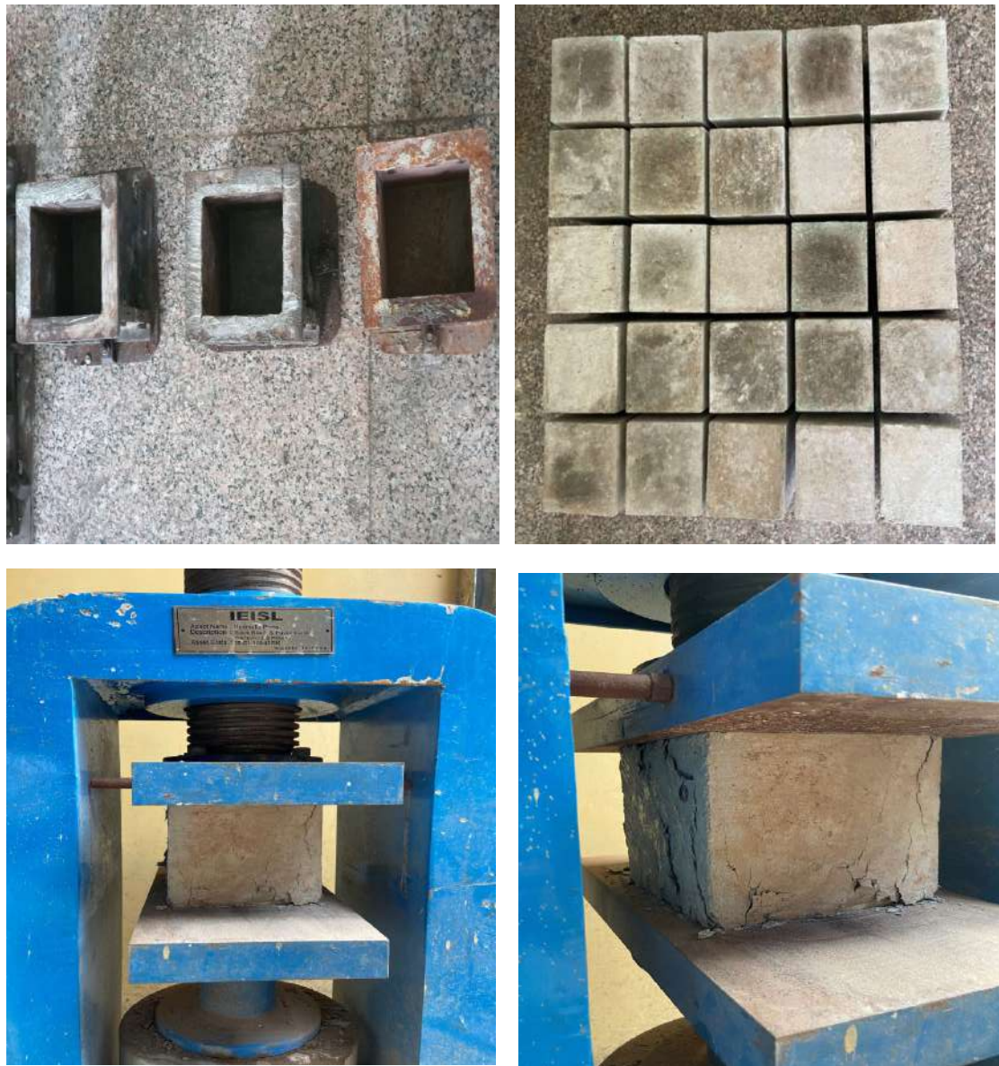
Figure 3.11 Compressive strength determinations
