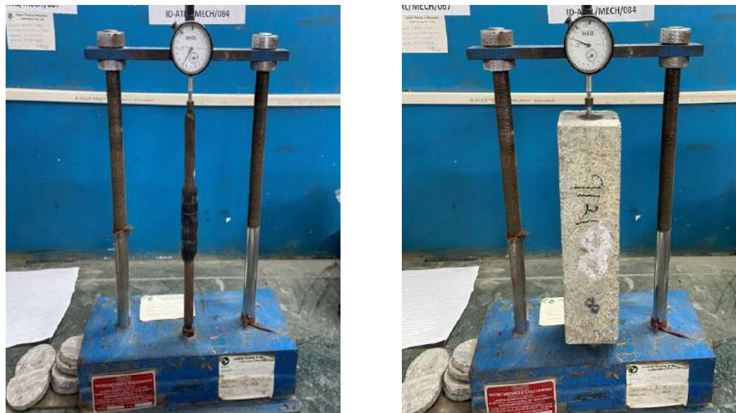
Figure 3.15 Drying shrinkage apparatus and specimen under testing
