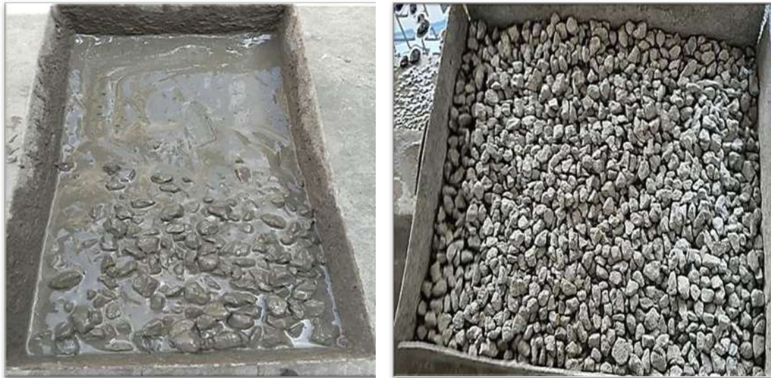
(a) RCA immersed in cement slurry (b) Cement slurry treated RCA
