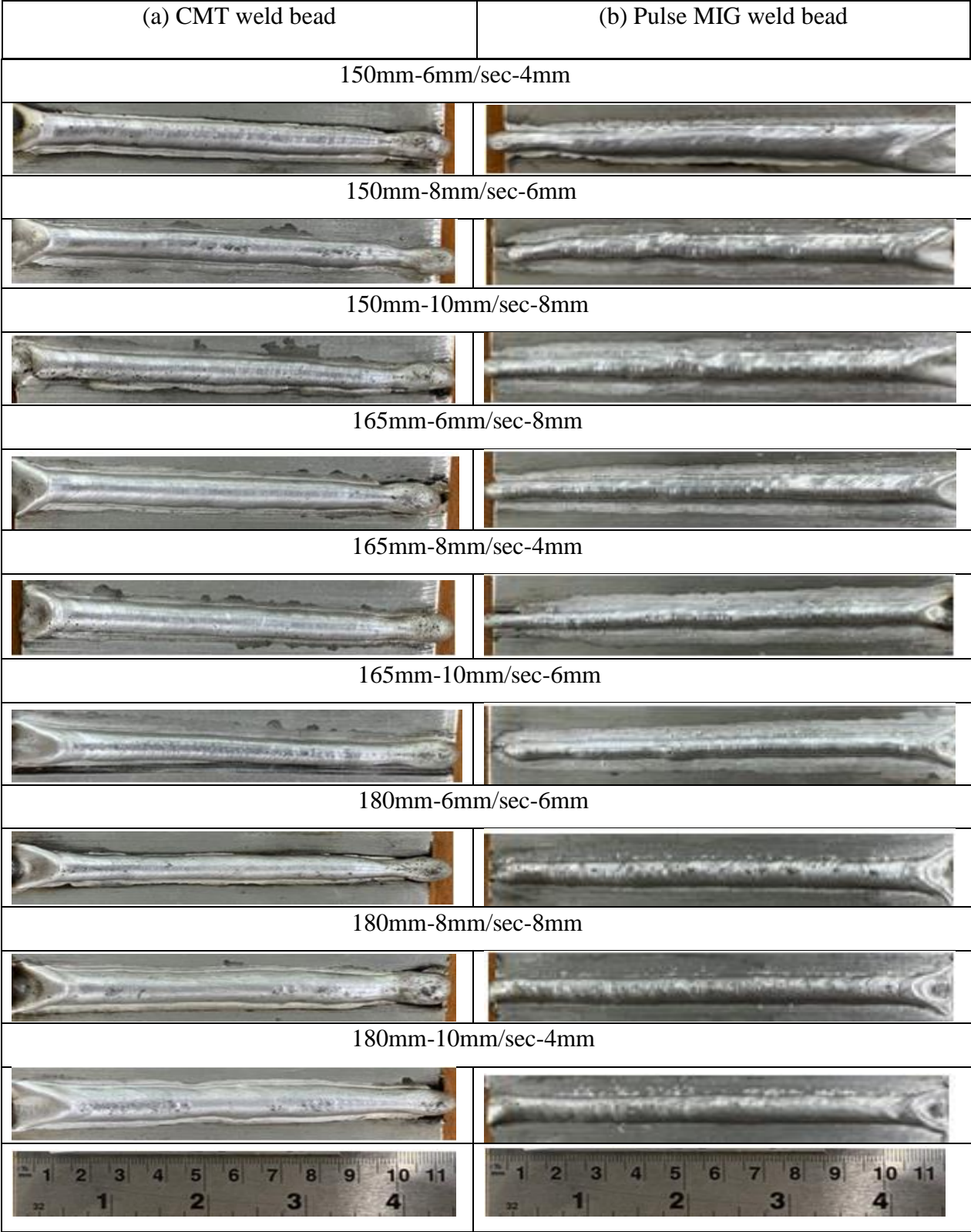
Figure 3.11 Weld bead images of (a) CMT and (b) pulse MIG welding
