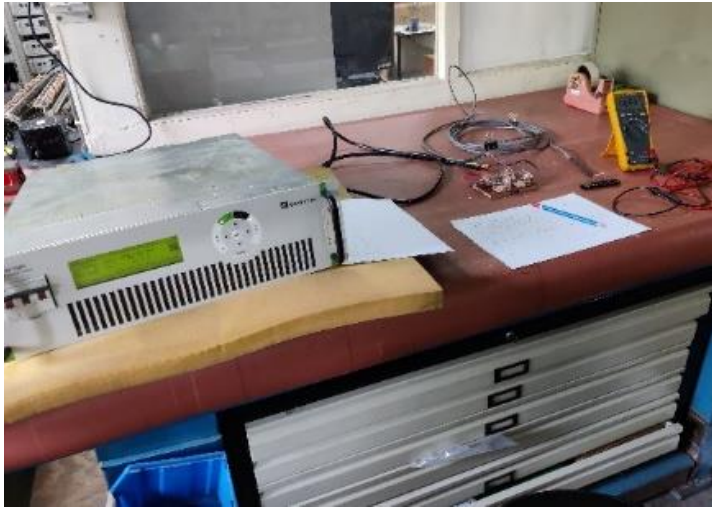
Figure 6.9 Test setup of the PCS diode assembly at room temperature (300 K).
