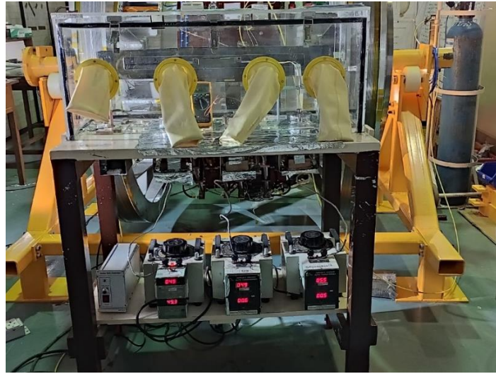
Figure 3.14 Joint-making station with argon hood.
