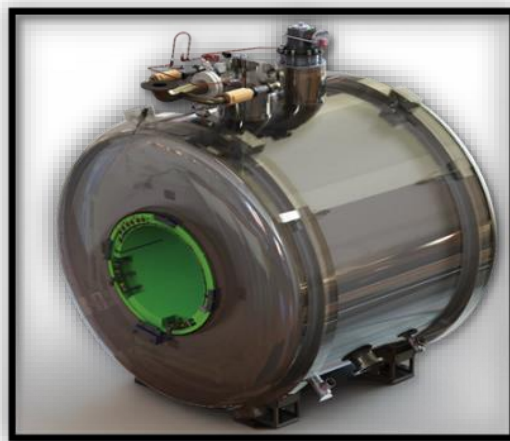
Figure 1.9 The 1.5 T superconducting magnet of IUAC.
