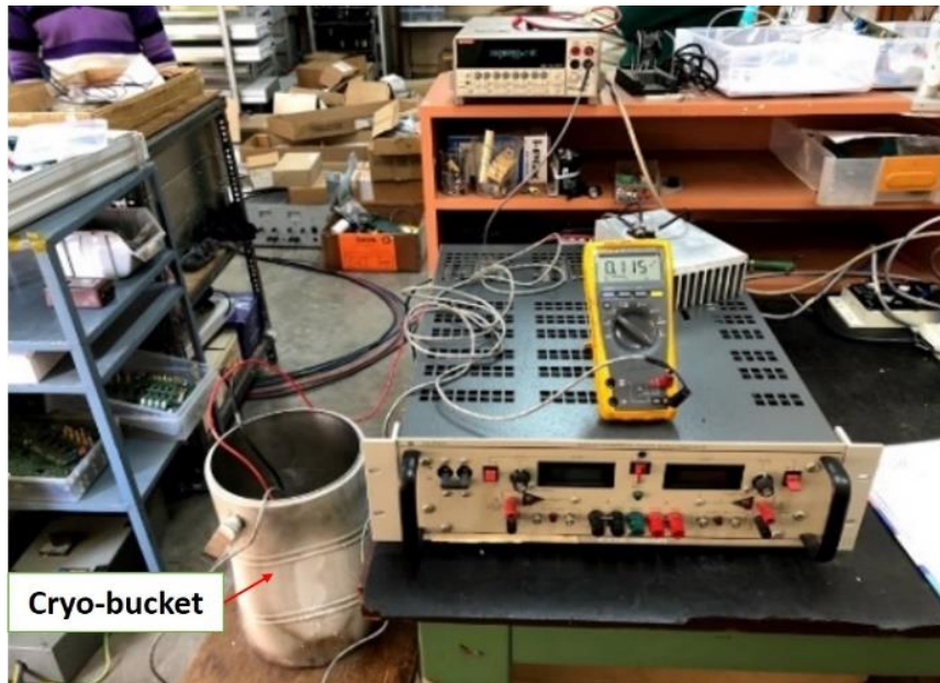
Figure 6.6 Photograph of the experimental test set up for the V-I characterization of diodes at 77 K.
