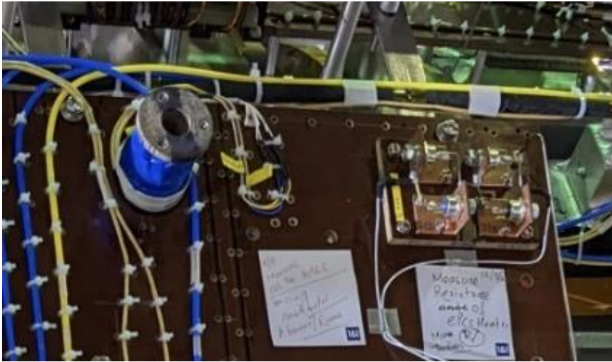
Figure 5.17 The PCS mounted onto the 1.5 T MRI magnet.
