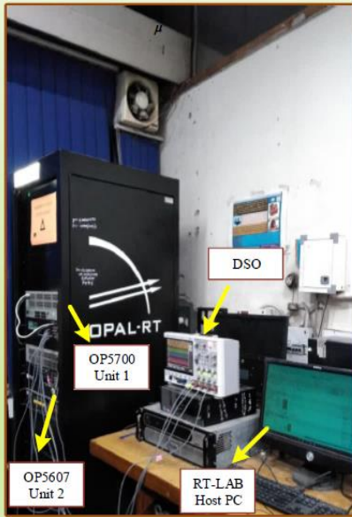
Fig. Real-Time Test Bench
