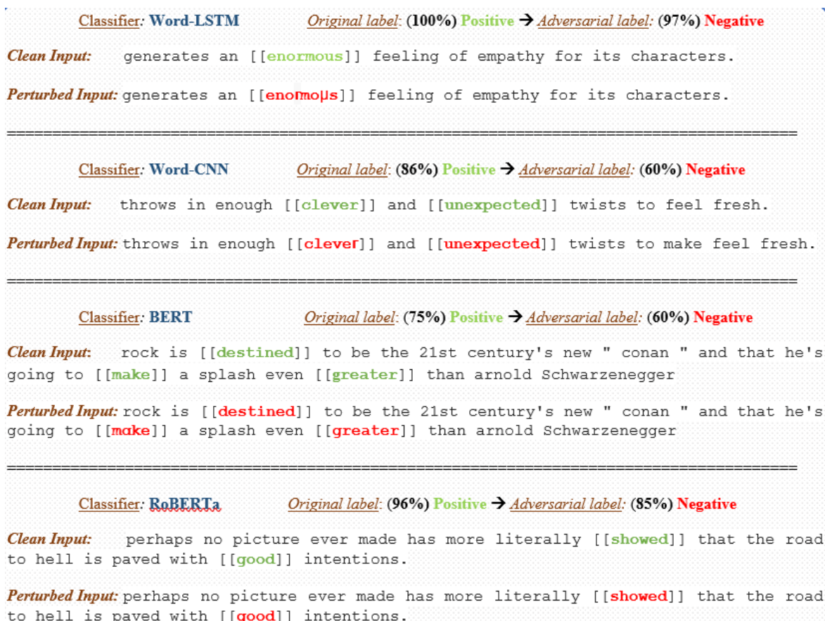
Figure 3.2 Adversarial Examples generated by replacing normal English characters with visually similar homographs
