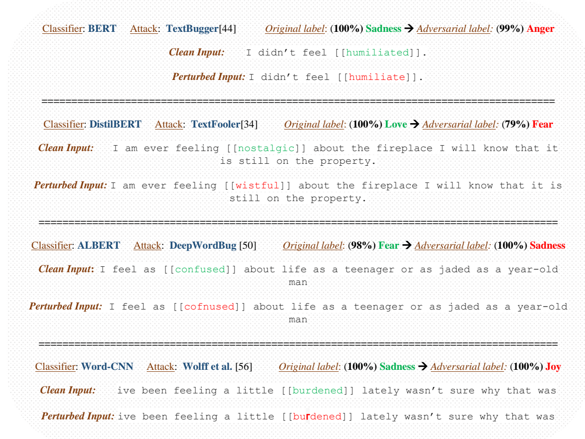
Figure 4.10. Adversarial examples generated through various word-level and char-level perturbation techniques
