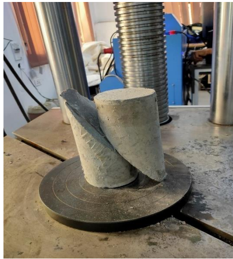
Fig. 4.21 Images show the slipping of two interfaces of cylindrical sample at peak level of load
