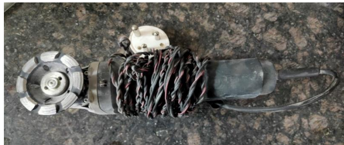
Fig. 4.8 Grinding machine used for leveling of surface
