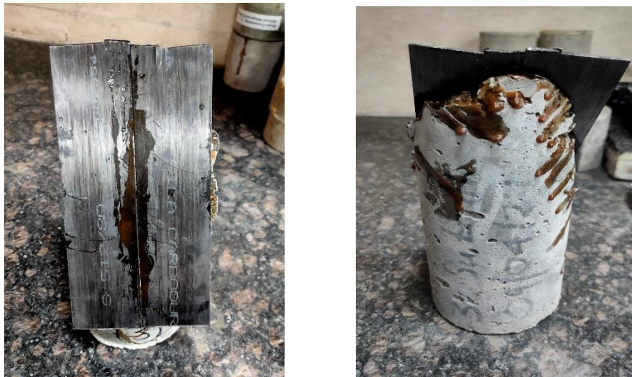
Fig. 4.14 Image representing complete fixation of FRP sheet to concrete surface The material properties of FRP as shown in Table 4.5 is provided by the manufacturer is used in the numerical validation of data later.
