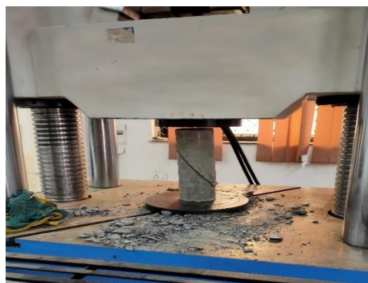
Fig. 4.20 Placing of cylindrical sample in the UTM for testing
