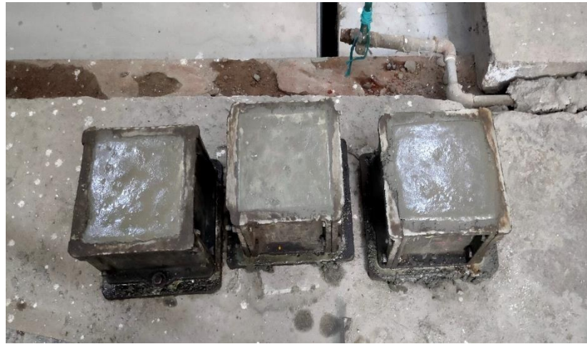
Fig. 4.16 Concrete mix filled in cubical molds
