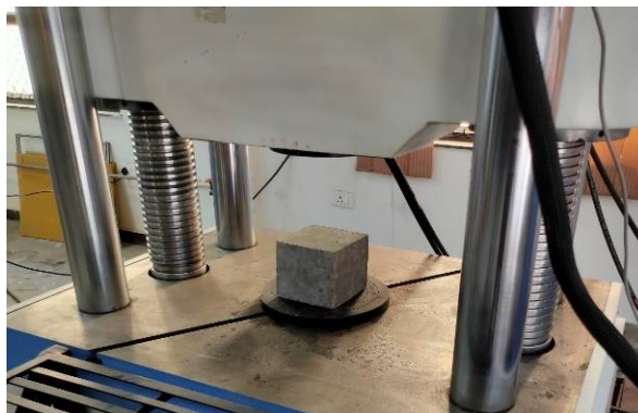
Fig. 4.18 Placing of concrete cube sample in the UTM for testing
