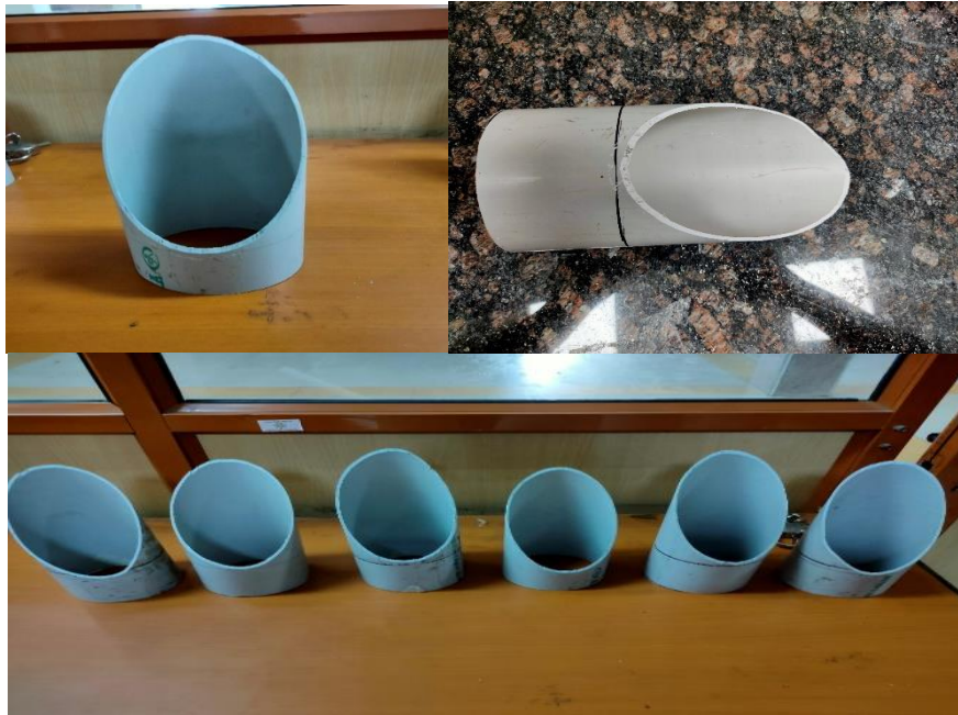
Fig. 4.5 Image showing the different orientation of molds prepared from the PVC Pipe
