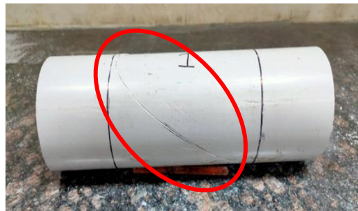
Fig. 4.3 Marking done on the PVC pipe
