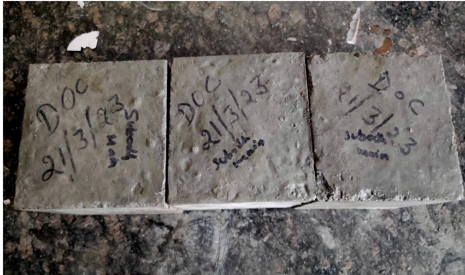
Fig. 4.17 Concrete cubes taken out of curing tank for testing
