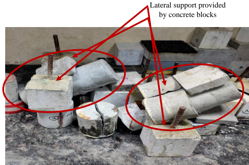
Fig. 4.15 Complete assembly to provide lateral and longitudinal support to cylindrical specimen
