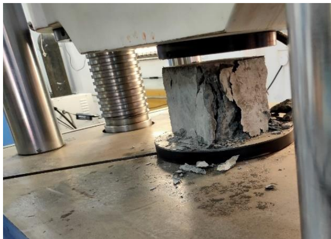
Fig. 4.19 Crushed Concrete Sample
