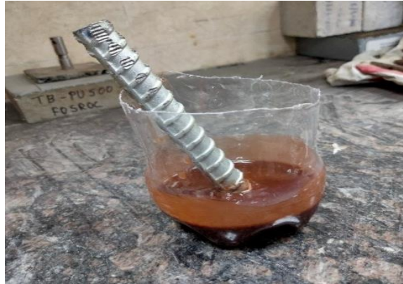
Fig. 4.12 Manual mixing of two parts of Epoxy
