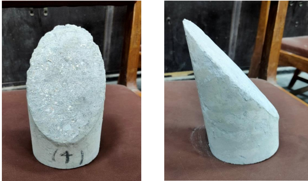
Fig. 4.10 Surface obtained after grinding operation
