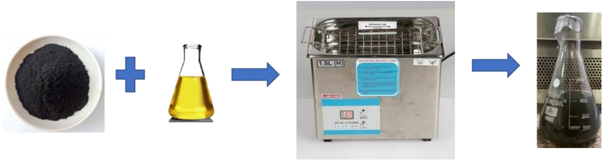
Fig. 3. 25 Blending of Pilot fuel with nanoparticles via Ultrasonicator
