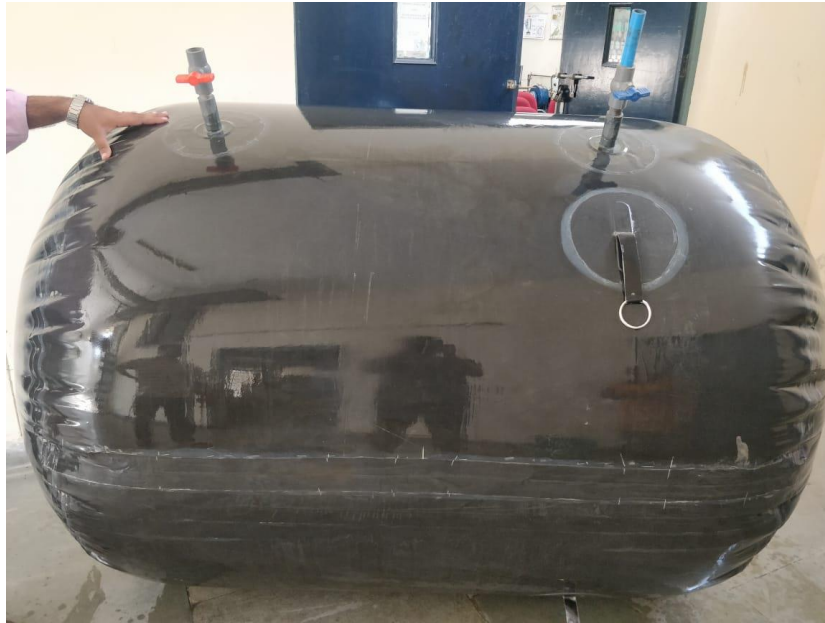
Fig. 3. 19 2 m 3 biogas storage balloon
