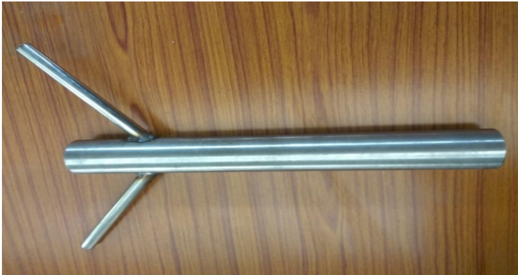
Fig. 3. 16 Illustration of the fuel-air mixing chamber
