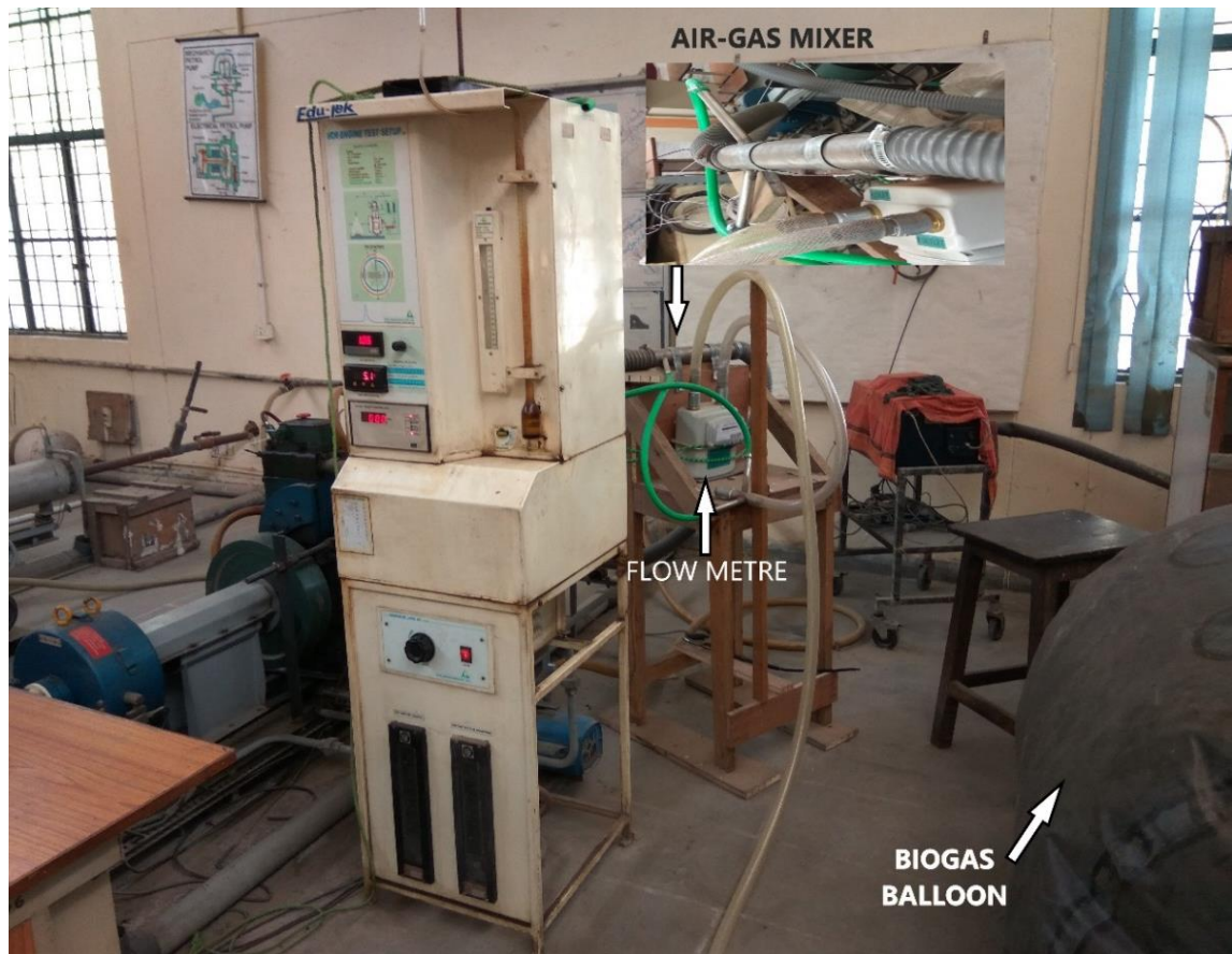
Fig. 3. 14 Pictorial representation of test rig after modification
