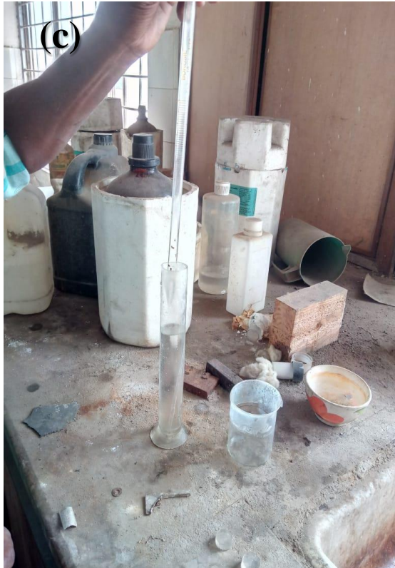
Figure 4.10: (a, b) polishing on emery paper and emery cloth, (c) making etching solution
