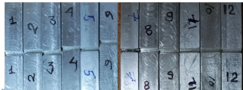
Figure 3:15 Charpy Test specimen as per ASTM Standard
