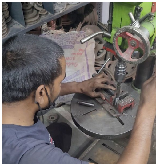
Figure 8.15 Chamfering metal piece using the drill press
