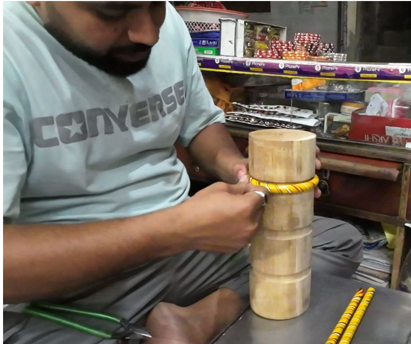
Figure 8.28 Placing shellac into grooves
