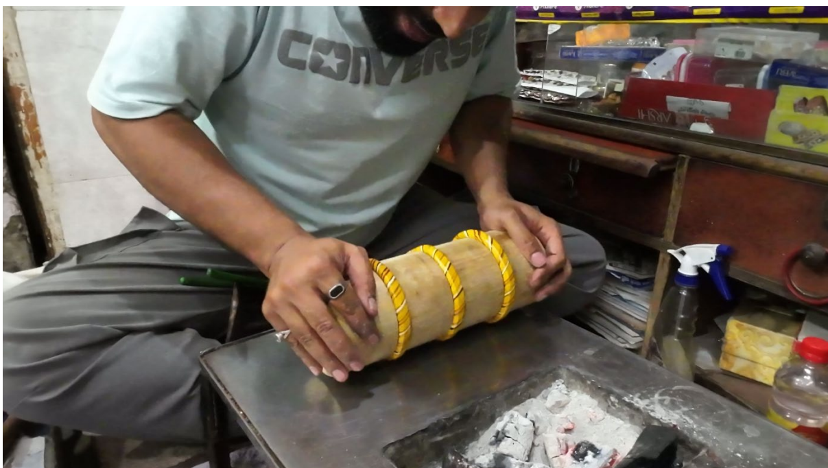
Figure 8.31 Rolling the lamp body on flat steel workstation
