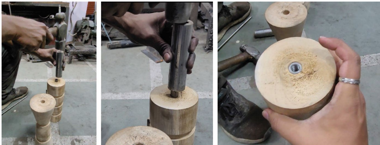
Figure 8.18 Hammering metal insert
