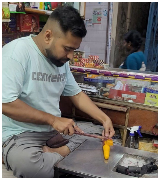
Figure 8.20 Adding yellow pigment onto shellac base
