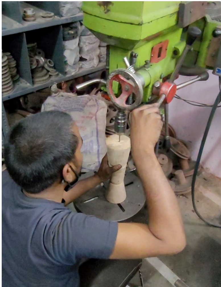
Figure 8.7 Drilling using a drill press
