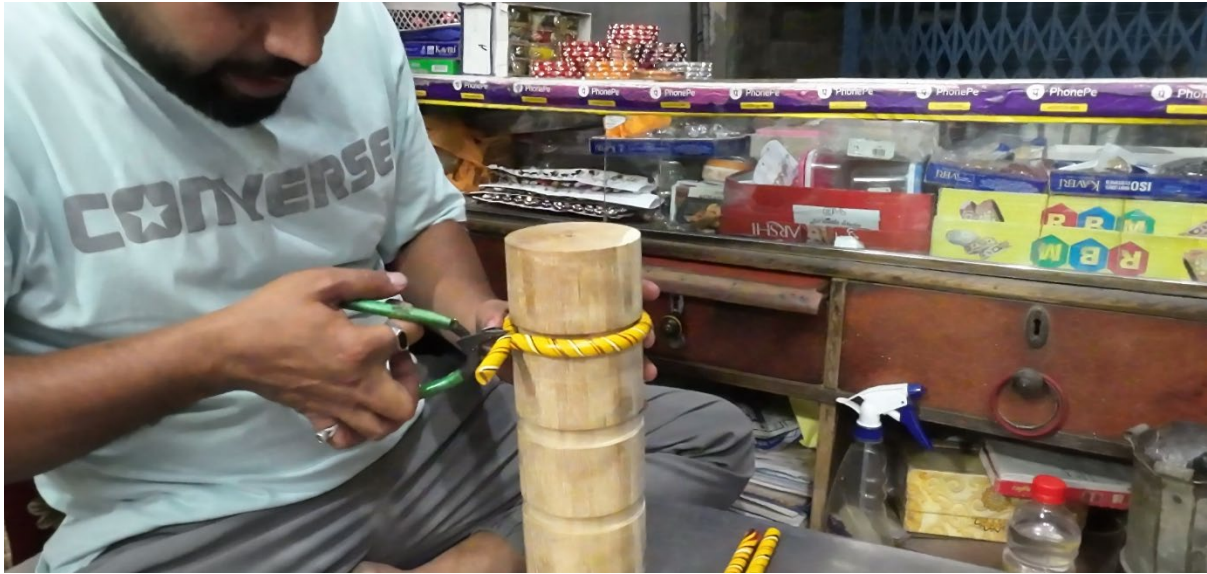
Figure 8.26 Cutting excess shellac part
