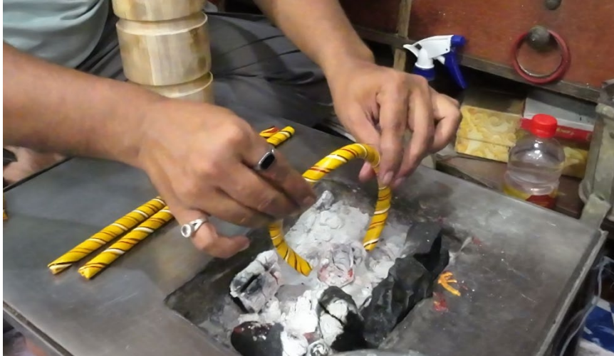
Figure 8.27 Heating shellac ends
