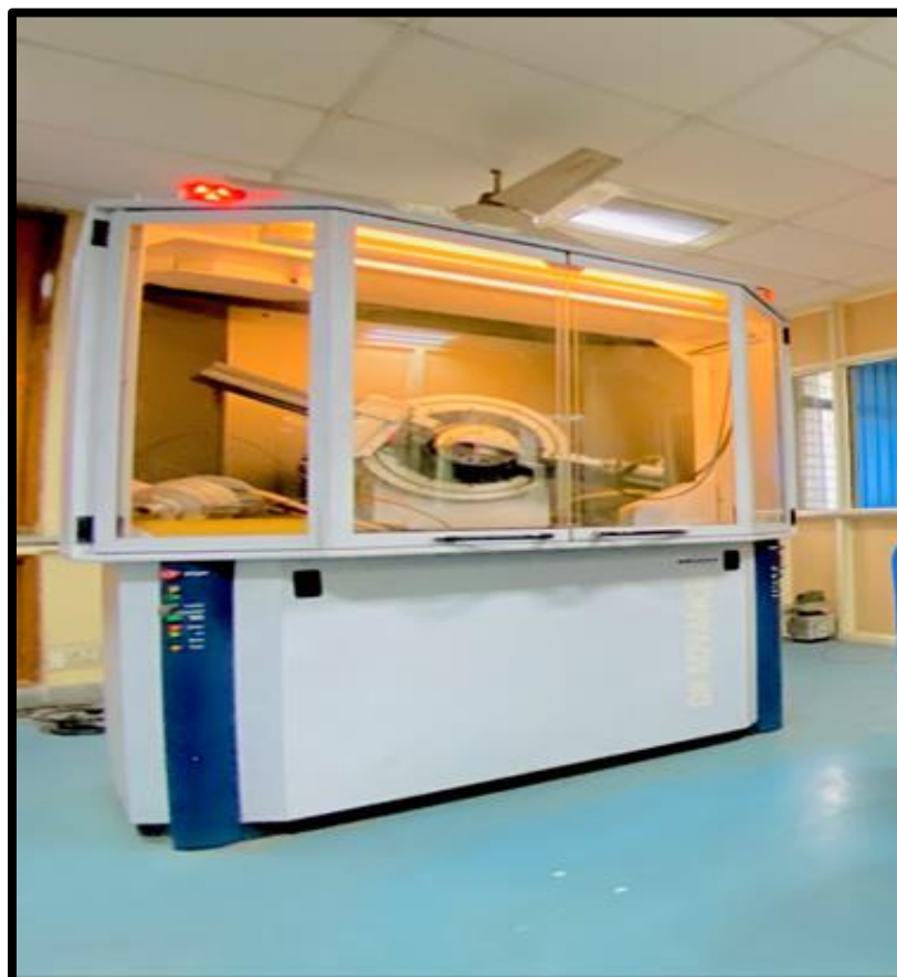
Fig. 2.2 Bruker D8 Advanced X-Ray Diffractometer.
