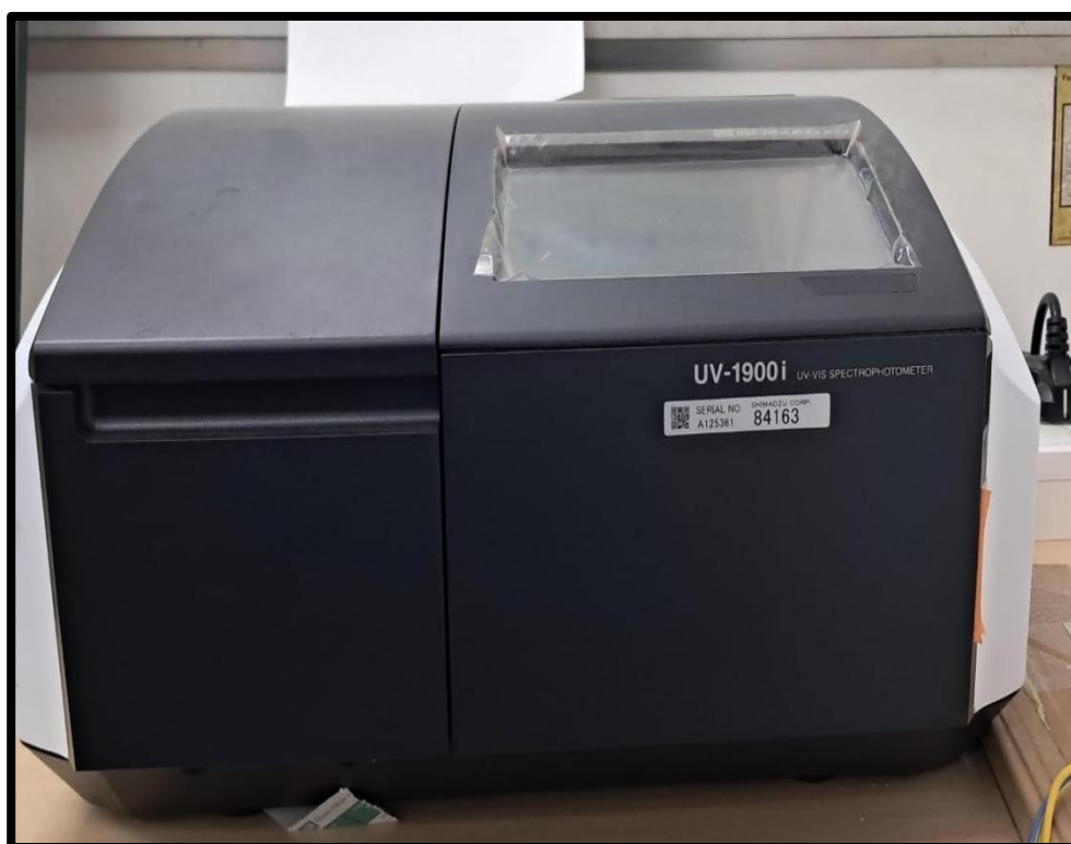
Fig.2.4: Shimadzu 1900 UV Spectrophotometer
