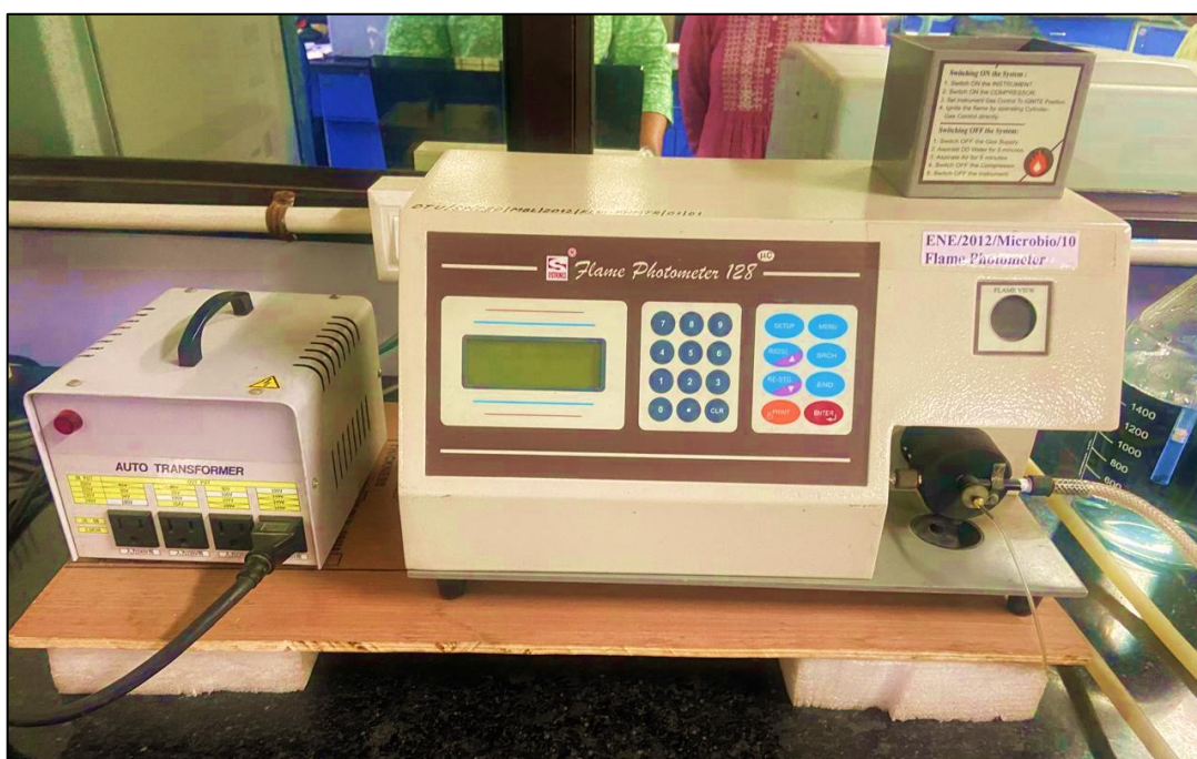
Fig 3.4. Flame photometer used for the analysis of cations ( \text{Na}^+ , \text{K}^+ , and \text{Ca}^{2+} )
