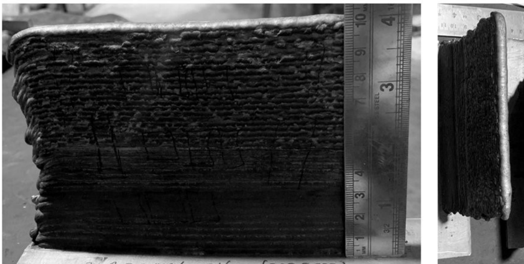
Fig. 4.14 The CMT WAAM Inconel 718 wall front view and top view with the optimized process parameters
