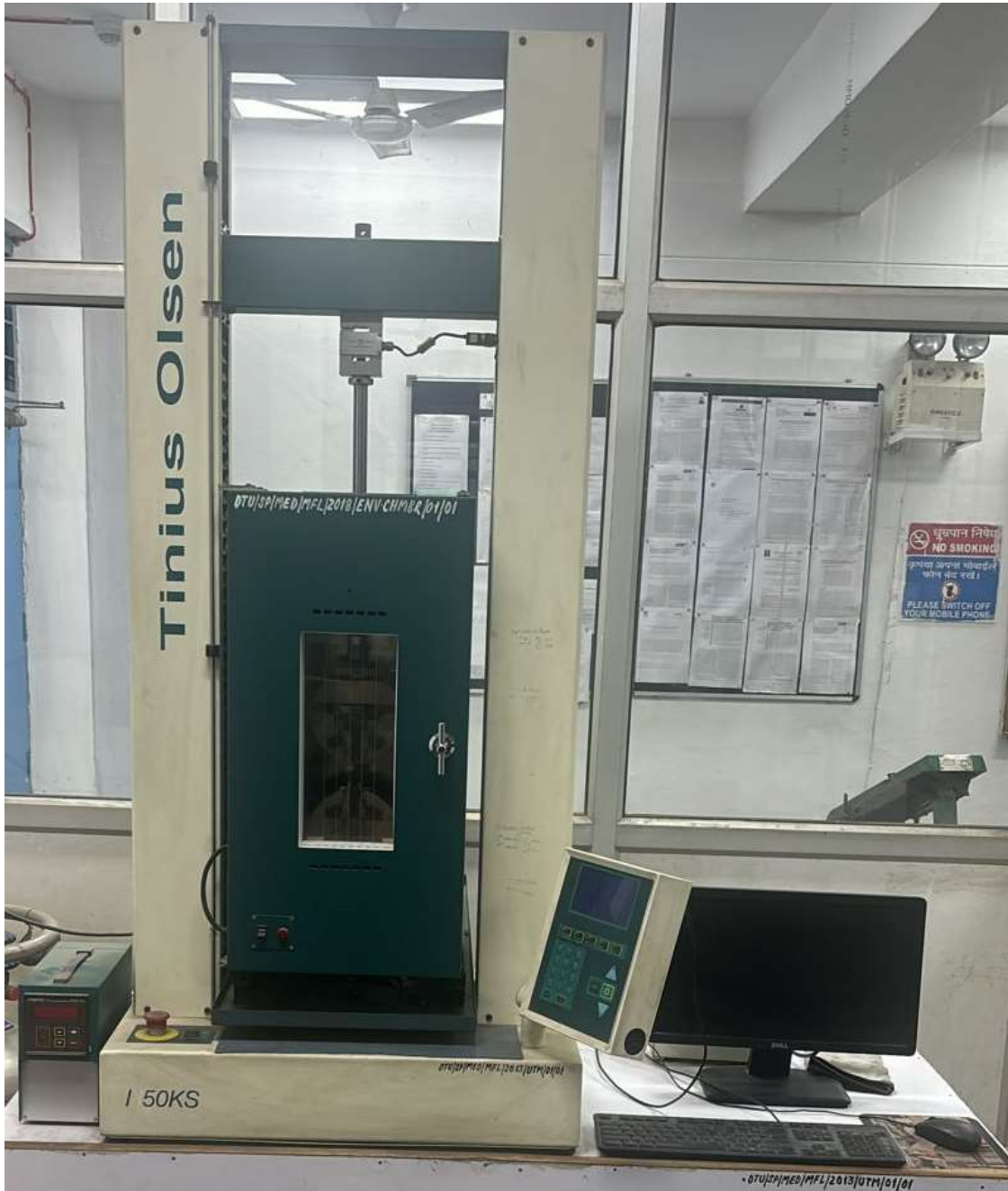
Fig. 3.7 Tensile machine (Model: Tinius Olsen H50KS)
