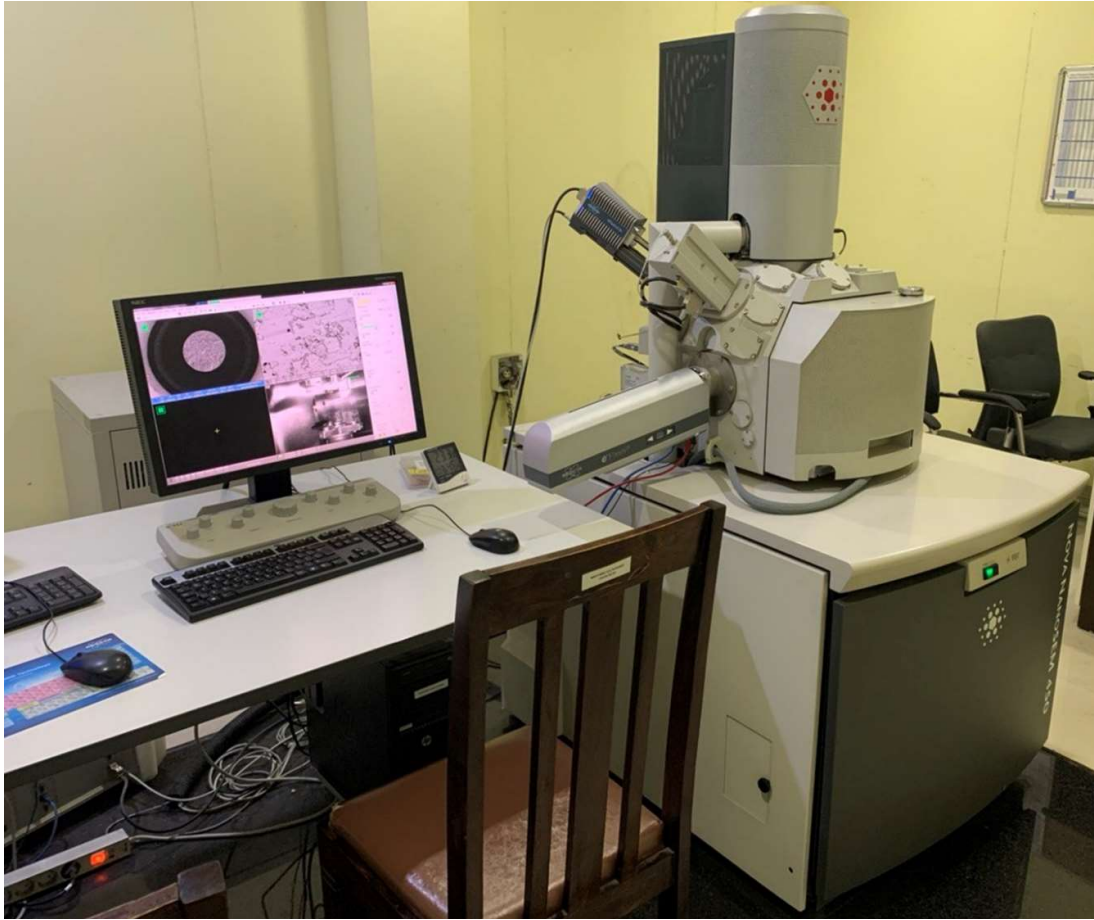
Fig. 3.9 Field Emission Gun Scanning Electron Microscope (Model-Nova Nano FE-SEM 450)
