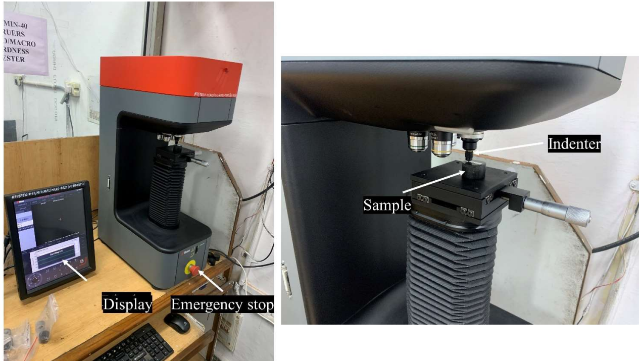
Fig. 3.6 Microhardness tester (Struers Duramin-40)
