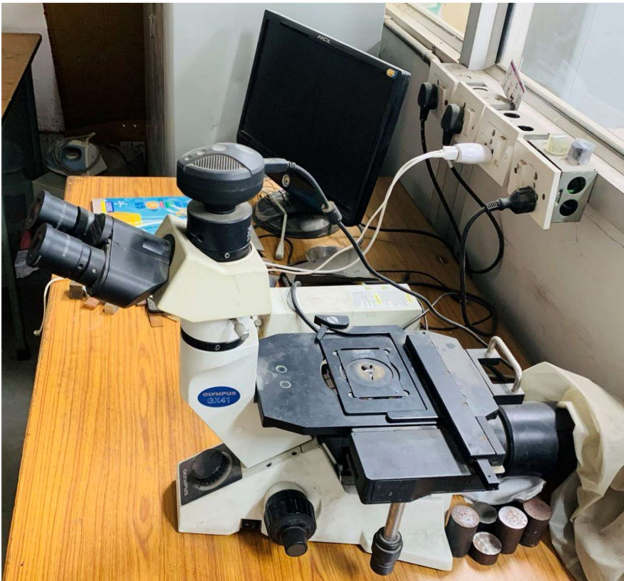
Fig. 3.8 Olympus GX41 compact inverted metallurgical microscope
