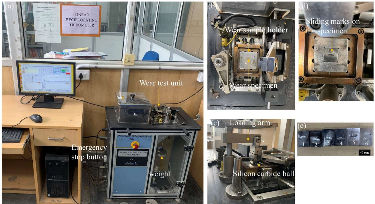
Fig. 5.13 (a) Linear Reciprocating ball on disk wear set up (b) wear chamber with sample holder and specimen (c) ball surface contacting the disk with load (d) sliding marks on disk surface (e) Worn out samples
