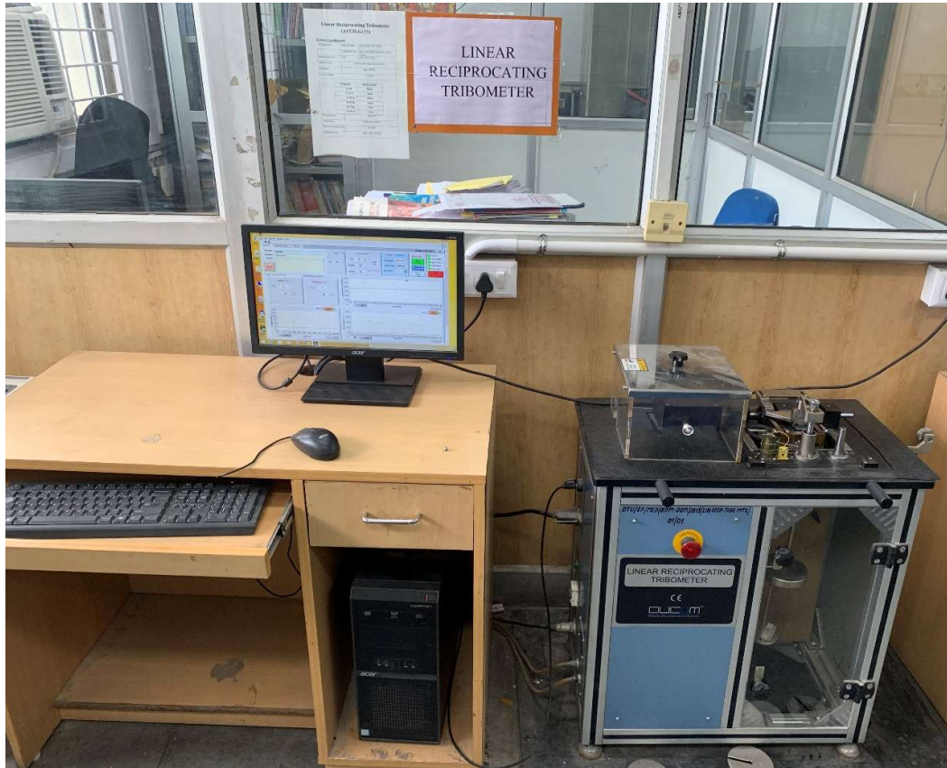
Fig. 3.11 Linear Reciprocating Tribometer (Model-Ducom)
