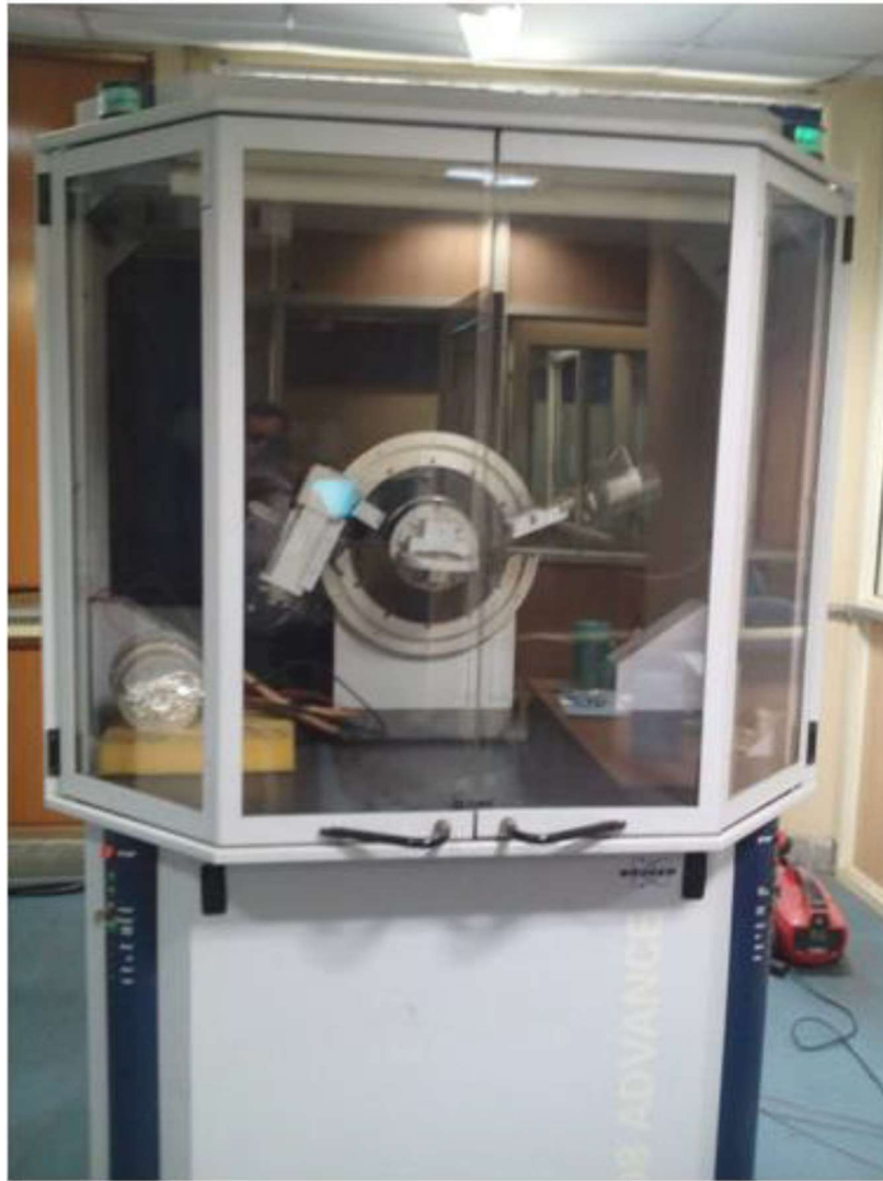
Fig. 3.10 XRD (Model: BRUKER D8 ADVANCED)
