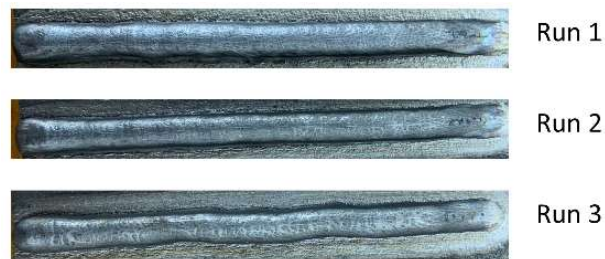
Fig. 4.13 Three weld bead images constructed on the optimum process parameters of IN 718
