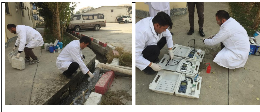
Figure 3. 4 Sample collection and field water quality testing.
