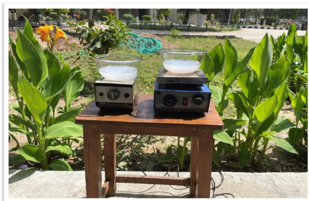
Fig. 3.2 Experimental setup of Solar-catalysis for degradation of CP
