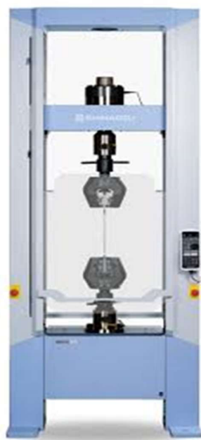
Fig. 3.1: Universal Testing Machine, Shimadzu, Autograph AG-X 110 N used for Tensile Strength and Percent Elongation at Break
