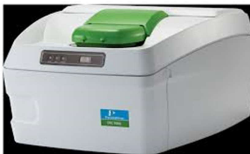
Fig. 2.5: Differential Scanning Calorimeter (DSC 8000, Perkin Elmer) used for Characterization of CMG Based Films
