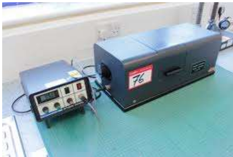
Fig. 3.6: Spherical Haze Meter, Diffusion Systems (M57d) used for Haze and Transparency
