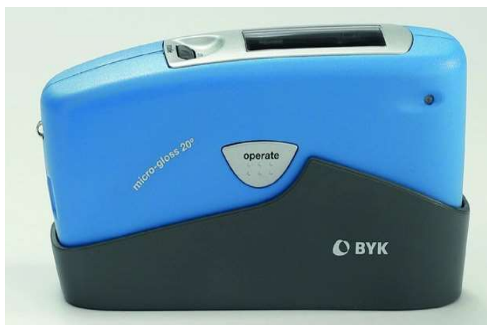
Fig. 3.5 Gloss Meter Model BYK Gardner used for Gloss Measurement
