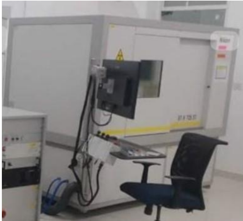
Fig 3.8 Nikon XTH 225 ST X-ray CT Scanner
