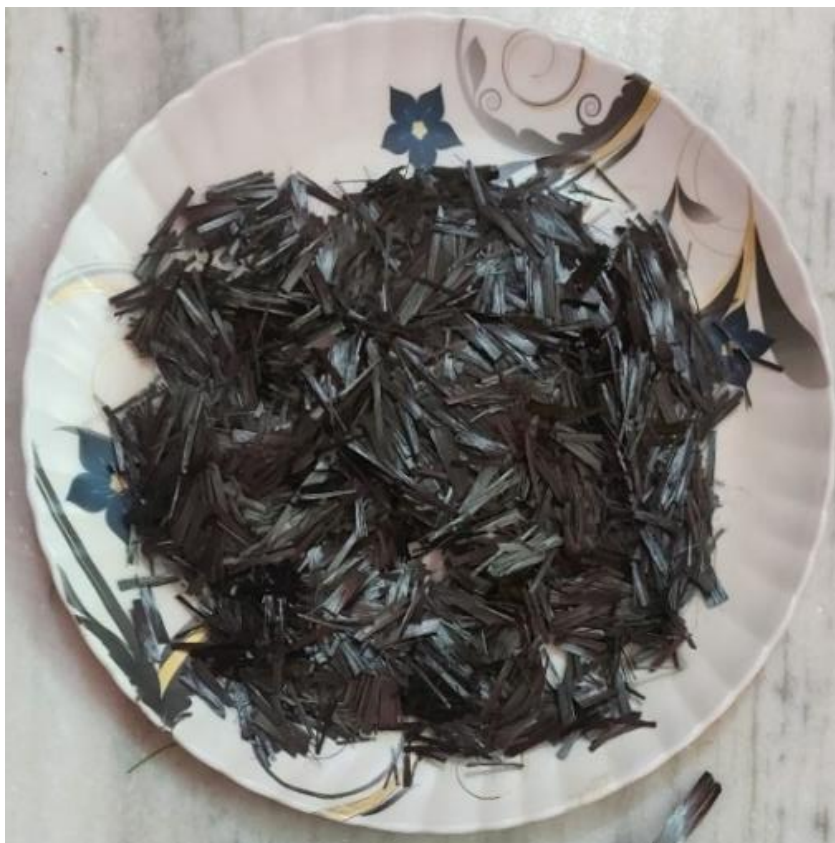
Fig.3.2 Carbon fiber with 25 mm length
