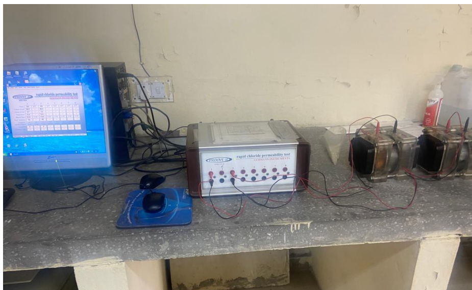
Fig.3.6 RCPT test setup
