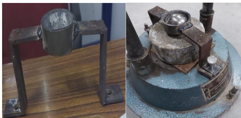
Fig.3.5 Adapted Instrumentation for the Drop Weight Impact Test
