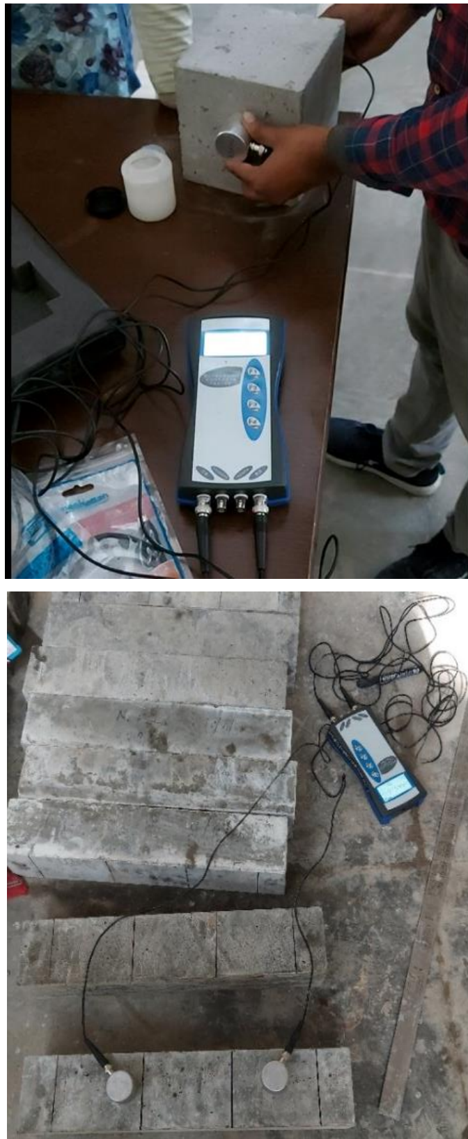
Fig.3.4 Ultrasonic Pulse Velocity Test Setup
