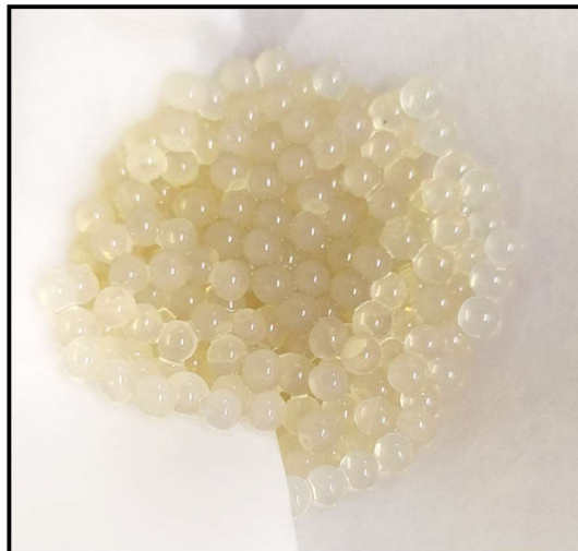
Fig. 3.31 Immobilization of P. oxalicum PBG30 phytase in calcium-alginate beads
