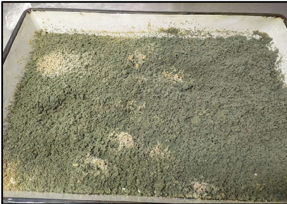
Fig. 3.16 Phytase production on a large scale in enamel-coated trays
