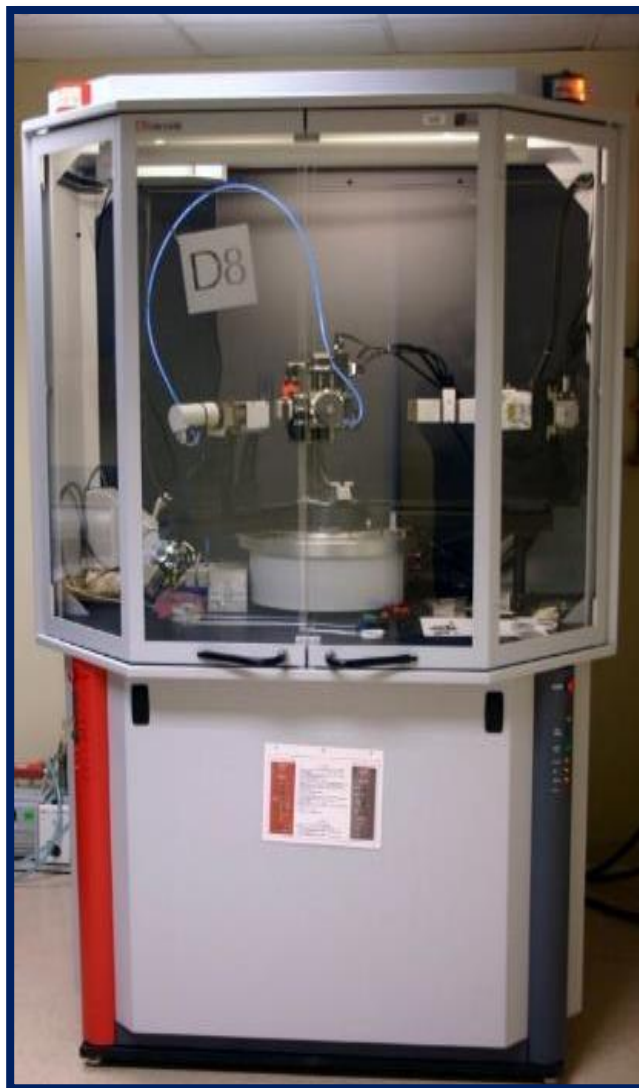
Fig.2.3: Bruker D8 Advance X-ray diffraction machine.
