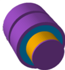
Figure 2.1 3-Dimensional structural view of DMGSE-JAM-CSG MOSFET.
