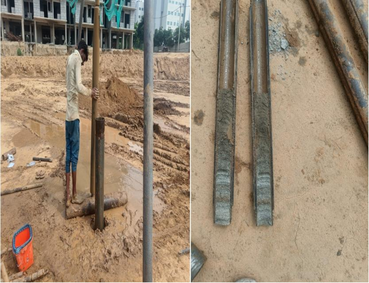
Figure 4.2 (a) SPT field set up and (b) Split spoon sample
