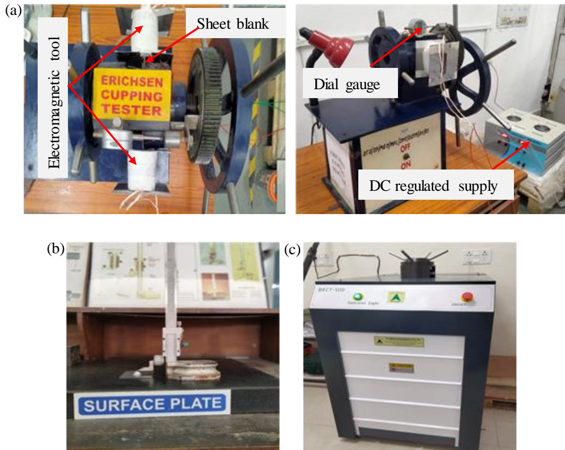
Figure 4.8 (a) Erichsen cupping experiment setup with MF, (b) vernier height gauge for IE value measurement, (c) BECT-100 Erichsen tester (IIT Roorkee) for force measurement.
