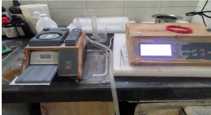
Figure 4.3 Electropolishing set up.
