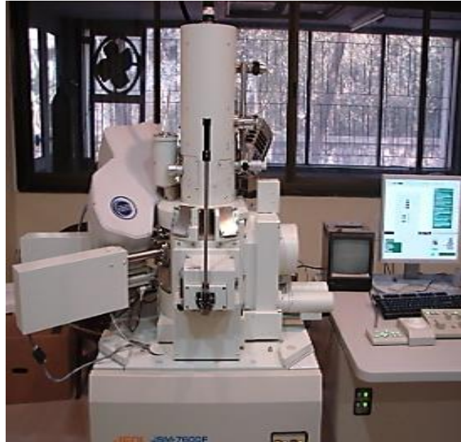
Figure 4.4 Field emission gun (FEG) scanning electron microscope (SEM) for electron backscattered diffraction (EBSD) analysis.
