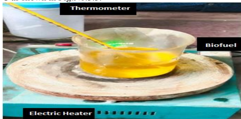
Fig. 3.3 Preheating of waste cooking oil
