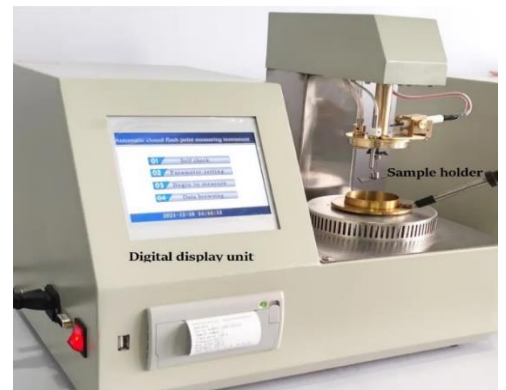
Plate 3.4: Flash point tester
