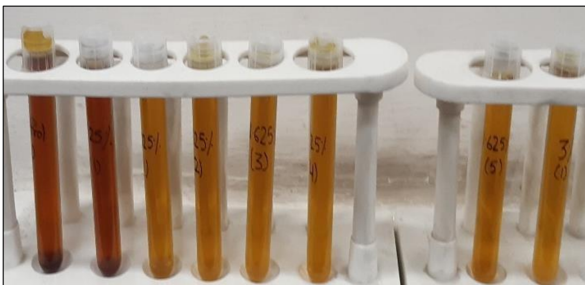
Figure 21. Sample test tubes of control, 0.25%, 1.625%, 3% NaOH (w/v) after 45 minutes of thermochemical pre-treatment.
