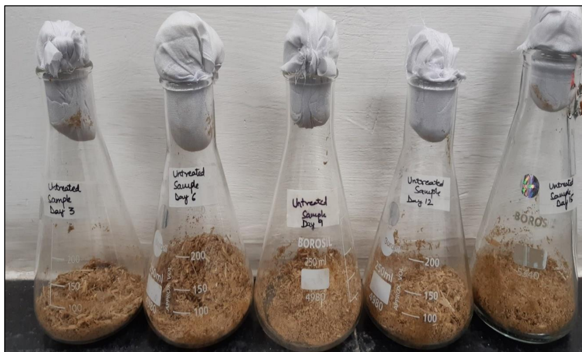
Figure 9. Solid state fermentation flask with untreated corn stover for different days of analysis.
