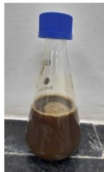
Optimized condition 3% NaOH, 15 minutes, liquid recovery
