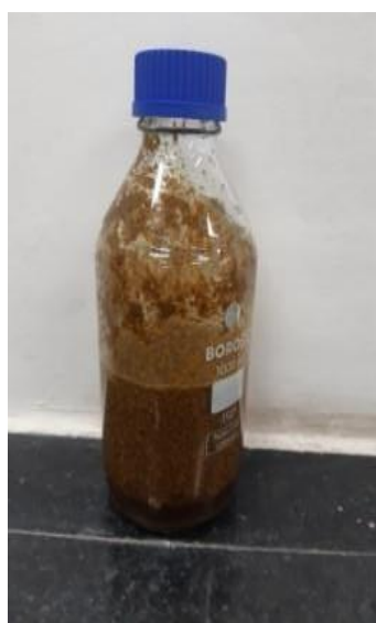
Optimized condition 3% NaOH, 15 minutes 50g in 500ml
