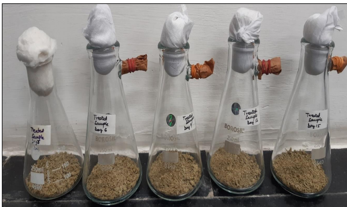
Figure 10. Solid state fermentation flask with alkali treated corn stover for different days of analysis.
