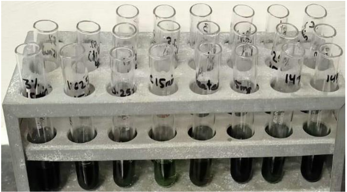
Figure 15. Sample test tubes after anthrone assay for cellulose estimation by Updegraff method.
