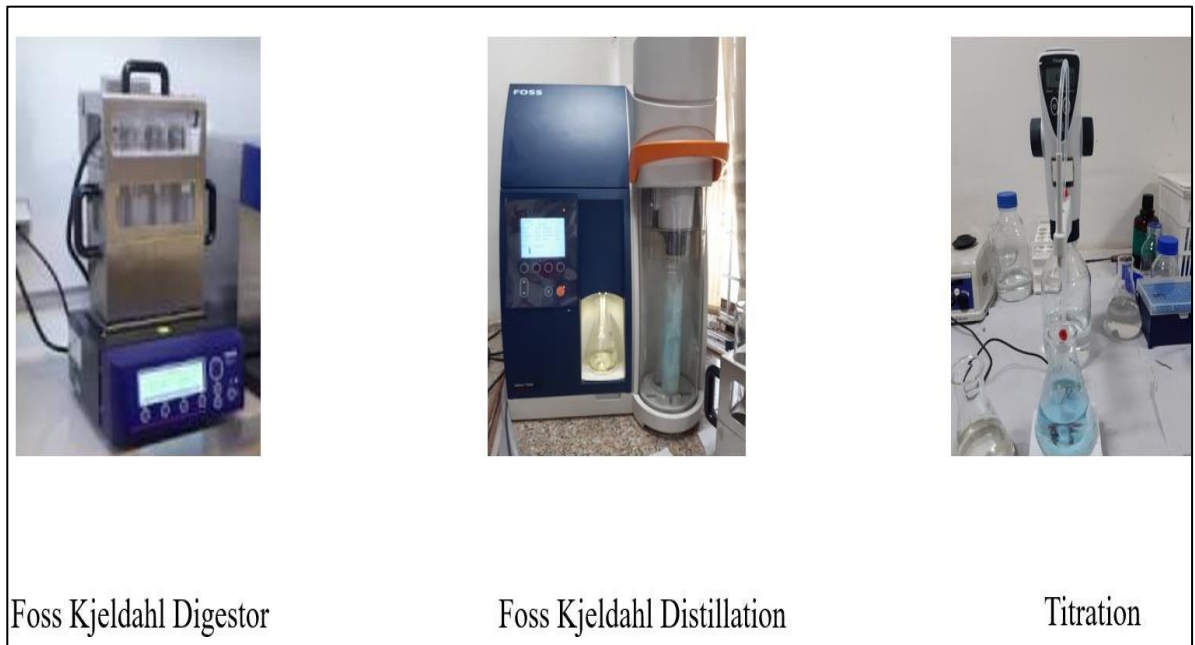
Figure 16. Protein and nitrogen estimation by Kjeldahl method involving digestion, distillation and titration method.
