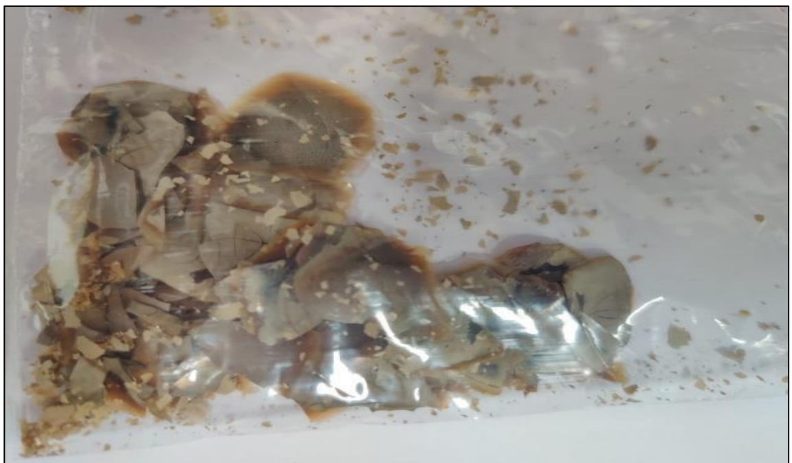
Figure 67. Microbial dry cell biomass recovery from modified media with hydrolysate for extraction of PHA after 48 hrs.
