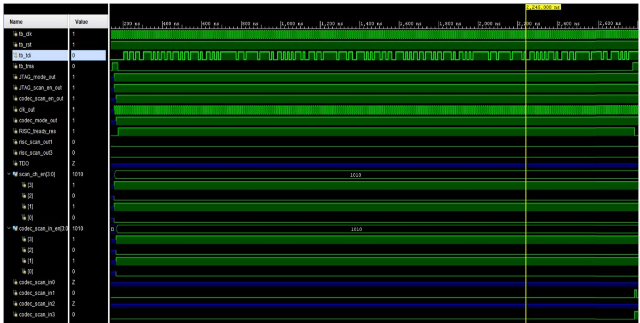
Fig 5.2: Simulation showing the loading of data register through TDI
