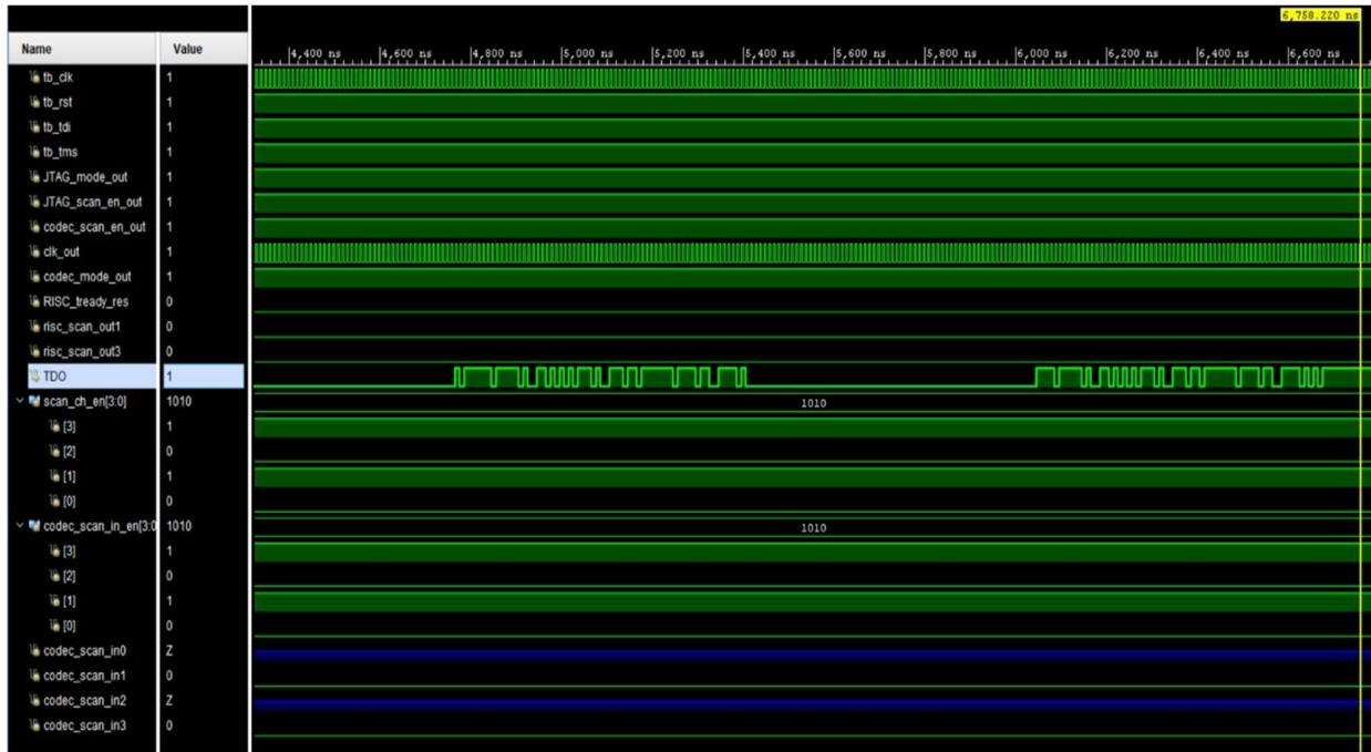
Fig 5.4: Simulation showing the serial transfer of response out from TDO
