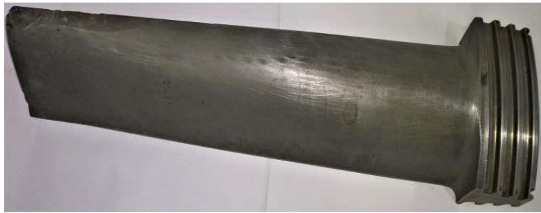
Figure 4.2. The edge of the turbine blade shows several pits/grooves
