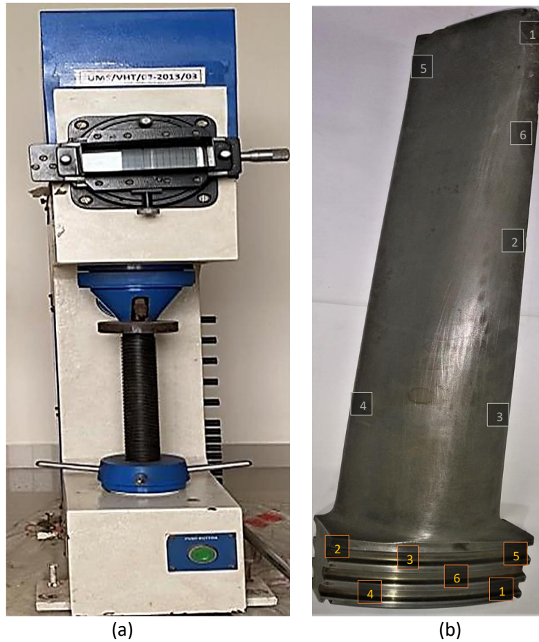
Figure. 3.10 (a) Hardness testing machine (b) blade profile and root hardness locations
