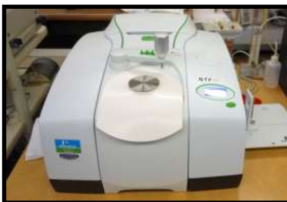
Fig.9-PerkinElmer Spectrum FTIR spectrometer
